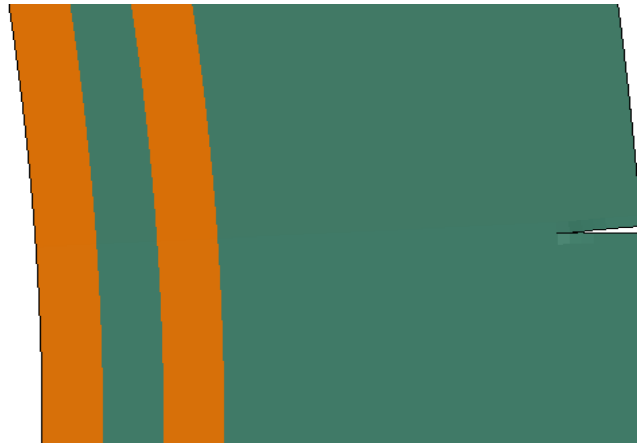
Figure 12. Partially Propagated Crack
