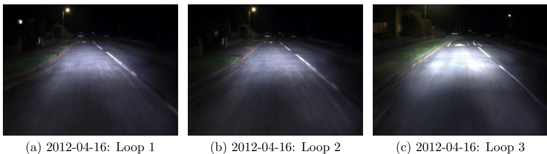
Figure A.3: Camera failure modes. The vehicle lighting and evening conditions combine to make this a very testing image sequence to perform VO on.
