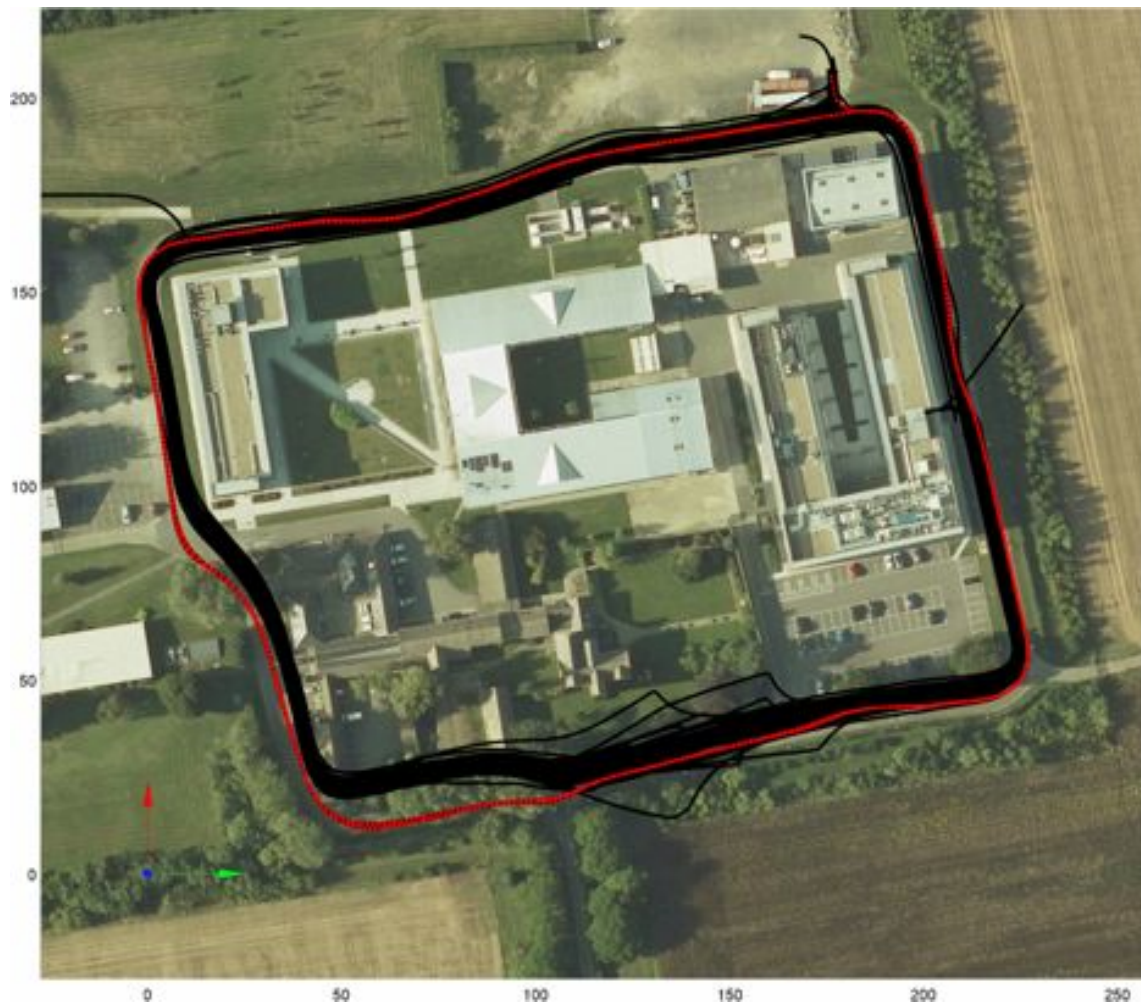
Figure 4.2: 26 kilometres of trajectory data around the Begbroke Science Park. A substantial dataset comprising of 3 months of INS data (26km total distance) around the Begbroke site in Oxford, contrasting areas of good GPS reception with poorer areas (predominantly the northern and southern sections). As can be seen in the lower section of the image, the trajectories exhibit a large variation, caused mainly by GPS signal degeneracy due to foliage. The majority of the trajectories (black, solid) are counter-clockwise, with a single clockwise loop (red, dotted).
