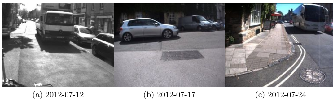
Figure 6.32: Woodstock town centre. An image sequence similar to Figure 6.31, but for the town centre. Again, note the large trucks in (a) and (c) - both sources of large velocity error. This compounded velocity error causes point cloud compression, which subsequently results in tracking failure.
