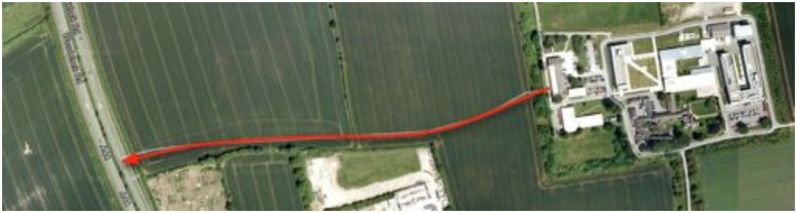
Figure 5.30: Featureless road section. A relatively featureless road section outside of Begbroke, described in Chapter 4. We use remission-based matching to stay localised in these areas.
