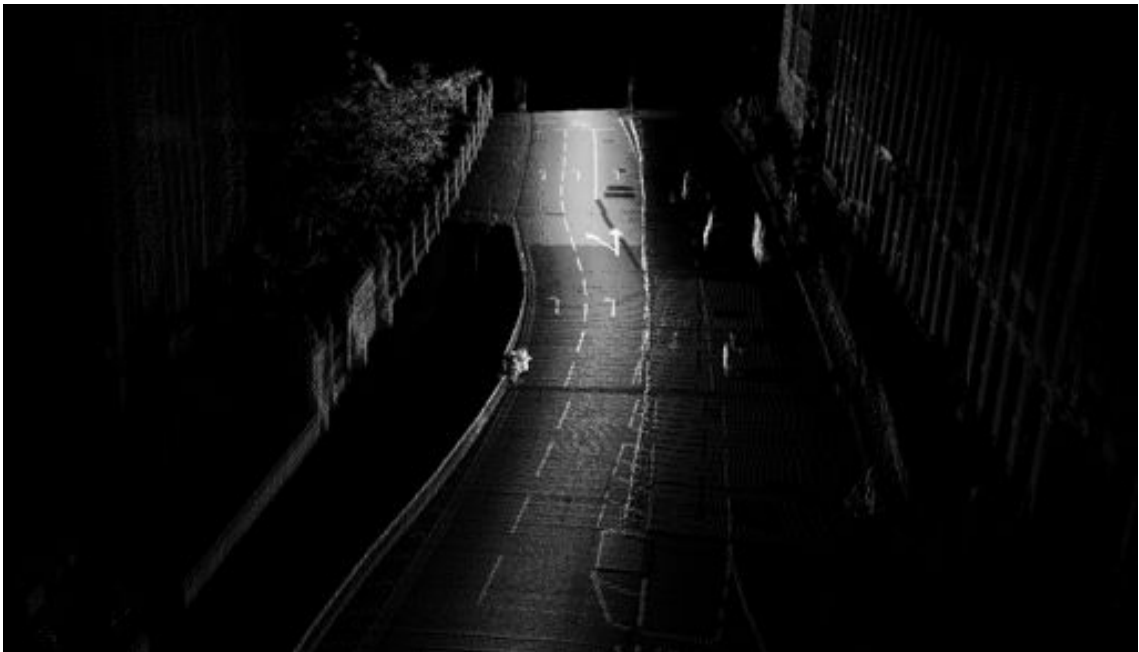
Figure 3.35: NABU dataset: Centre of London. An exemplar dataset collected by the NABU, driving past the Houses of Parliament - note the excellent reflectivity map. (Thanks to Ashley Napier for the point cloud data from this run)
