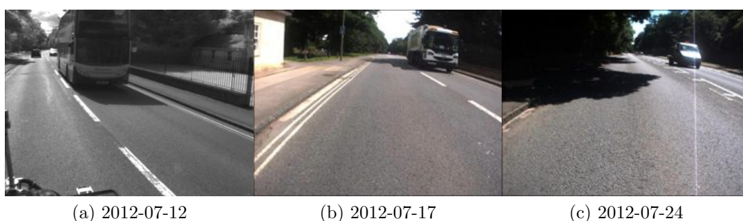
Figure 6.34: Woodstock exit. The final exemplar scene - the busy main road leaving Woodstock. The regular presence of buses (a), garbage-trucks (b) and other vans (c), all highly visible from the bumper-mounted LIDAR induce a large velocity error.
