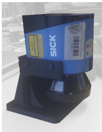
Figure 2.7: SICK scanning LIDAR. An LMS-151 scanning-LIDAR unit, used throughout this thesis. The unit in this image is mounted upside-down in a custom, rapid-prototyped mount.
