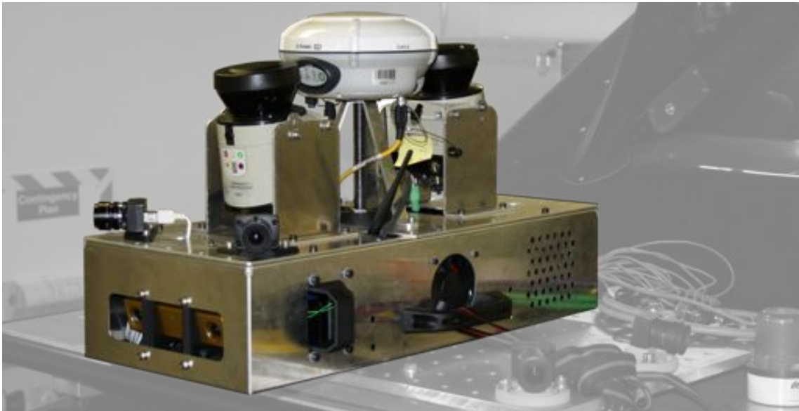
Figure 3.33: NABU: Mounted on the Wildcat. The NABU mounted on the MRG Wildcat. Visible are the PointGrey FireFly cameras (front-left, front-right), the SICK LIDARs (both inclined and declined) and the Trimble R8 GPS unit.
