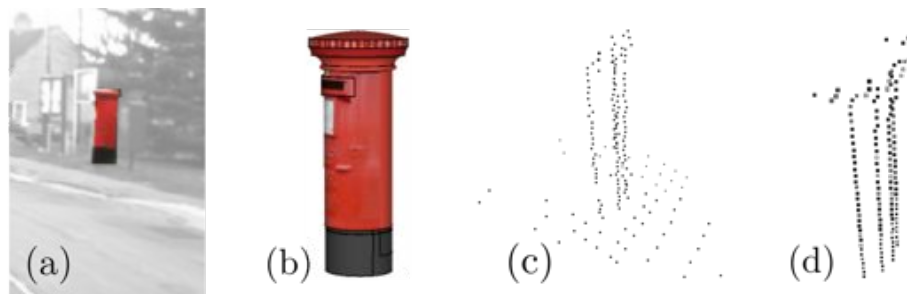
Figure 3.24: Commonly encountered: Postboxes. A regular sighting around English towns - free-standing postboxes (a), the CAD model (b), the real-world LIDAR data (c), and the simulated data (d).
