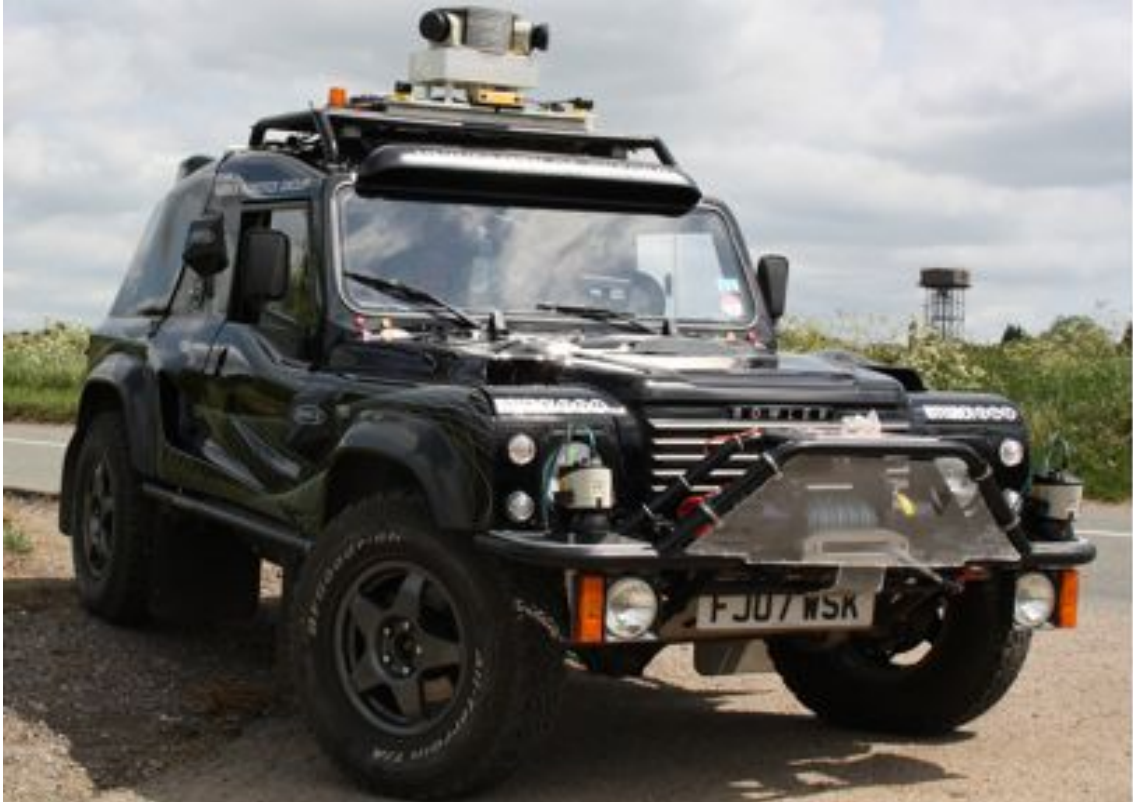
Figure 4.1: The MRG “Wildcat” . The Wildcat is a heavily-instrumented platform initially developed by BAE systems. The vehicle is equipped with an Oxford Technical Solutions Inertial Navigation System and a host of sensing modalities including LIDAR and camera units.
