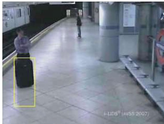
Figure 6. One example of object flagged as abandoned, although owner is nearby.
