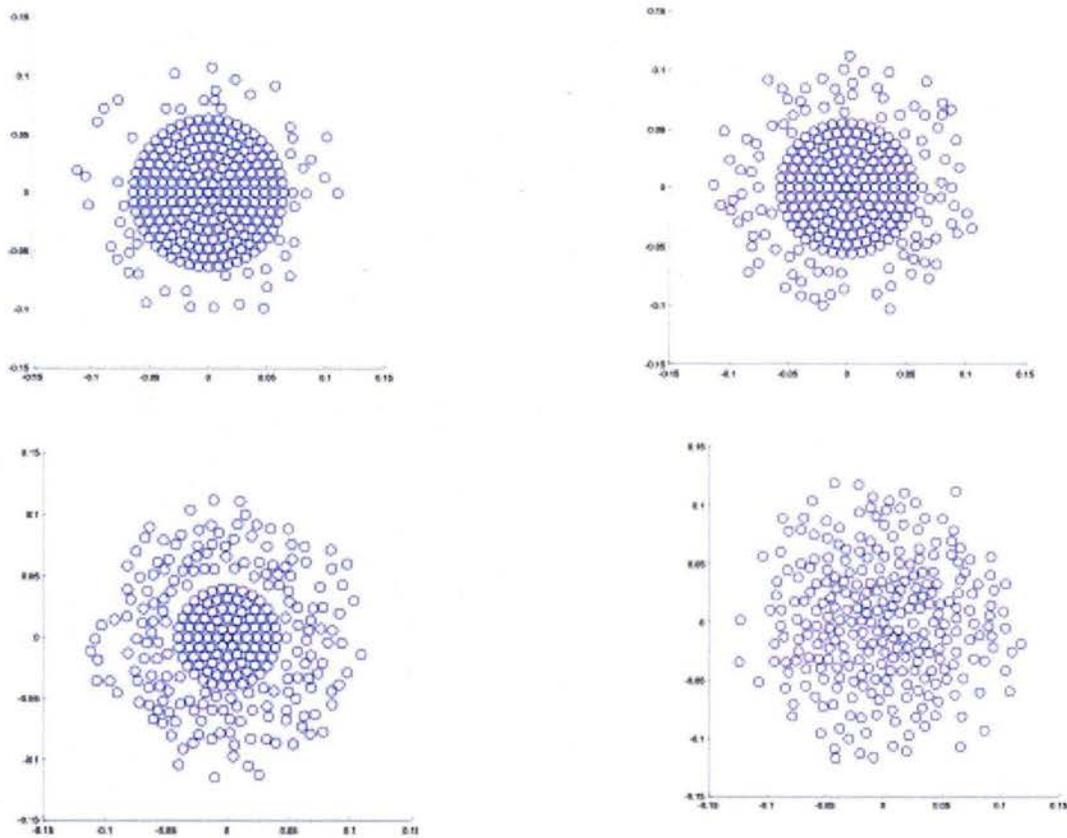
Fig. 1.2. The figure illustrates the stages in the generation of a nonuniform fiber distribution. The bottom right figure is the final configuration of fibers.
