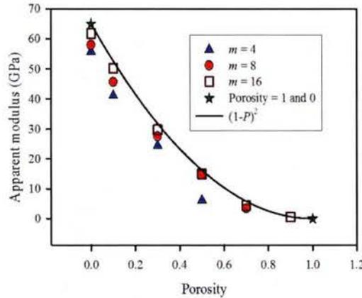
**Figure 2.1. The apparent modulus versus porosity for a IHPD model computed with different m-ratios (m=horizon size divide by the grid spacing). Notice that the results converge to the classical relationship for poroelastic materials.**
