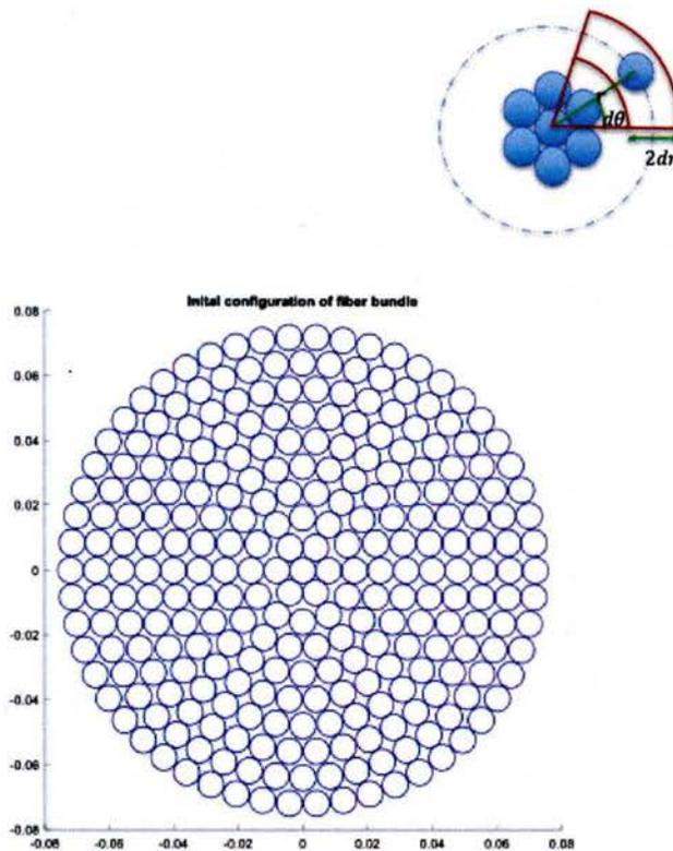
Fig. 1.1. A representative configuration of a dry fiber bundle is displayed in the figure to the left and the top figure shows the two variables  $r$  and  $\theta$  used in simulations to produce nonuniform configurations.
