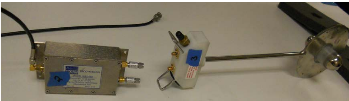
Figure 8. The balun (Prodyn Model BIB-105D) on the left connects to the D-dot sensor (Prodyn Model AD-40E®) on the right.
