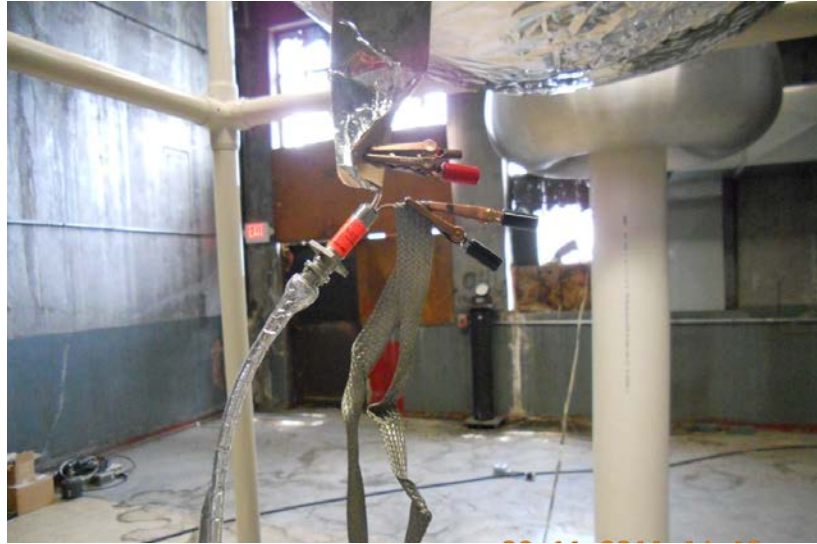
Figure 29. The CVR input and output terminals connect to the strike globe and the ground line respectively. The CVR signal is transmitted on a 25 ft shielded RG62 BNC cable. This configuration was in use while collecting the Table 7 data.
