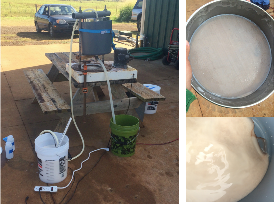
Fig. 12 Setup for sieving diatom cell walls on the left, metal sieve and final sieved cell walls on the right.
