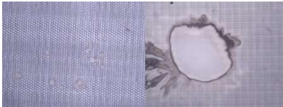
Figure 4 - CW damage morphologies of pure \text{TiO}_2 film (left) and nanolaminate film (right) at the same fluence [from Taylor and Talghader DEPS Symposium 2012]
