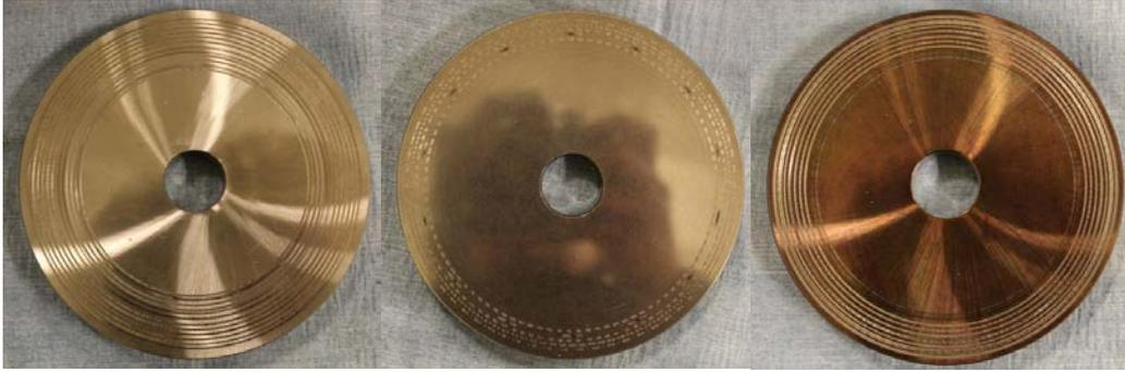
**Fig. 16 Images of the radially ground (left), ISF #2 (center) and black oxide (right) discs after experimentation**
