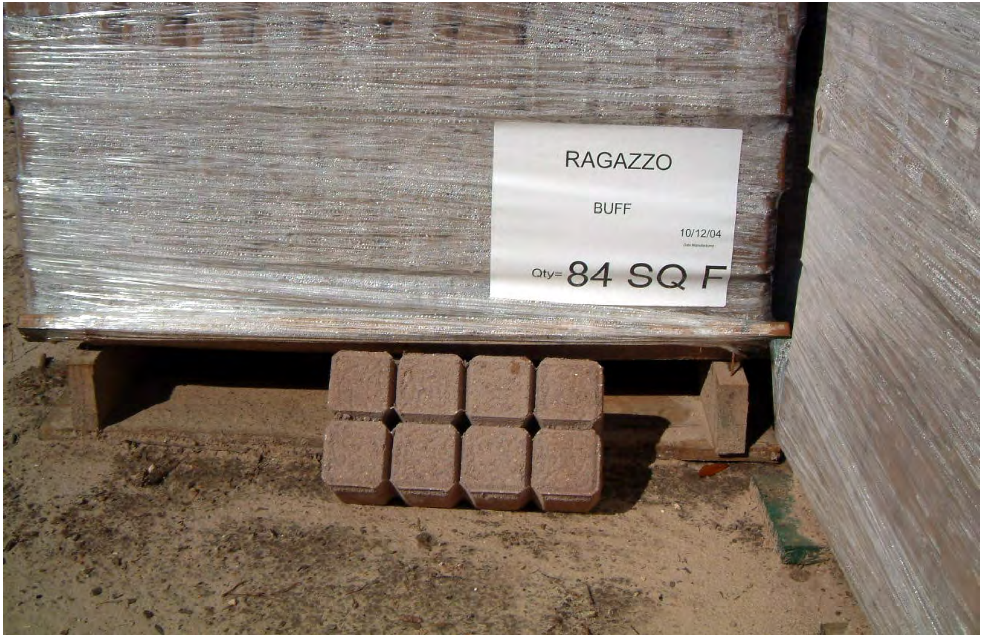
CONCRETE “RAGAZZO” BLOCK DETAIL MEASURING 6” W. X 12” L. X 3” DEEP
