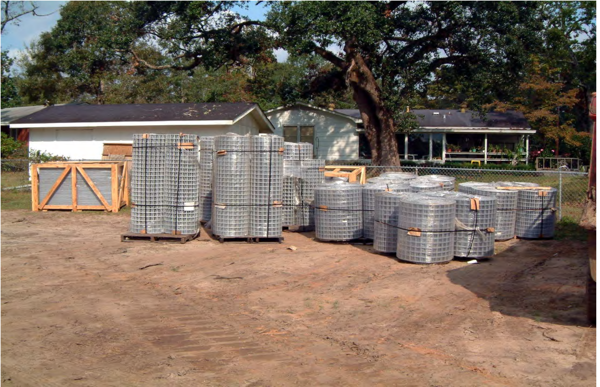
PVC COATED GABION MATERIAL IN “ROLL-STOCK” FORM
