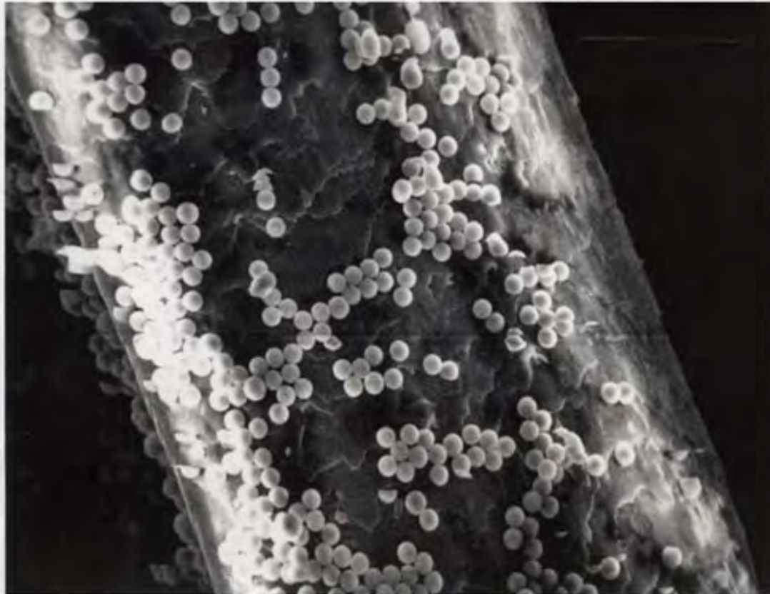
SEM PHOTO of 3.4 \mu m PARTICLES ON HUMAN HAIR, 1000X
