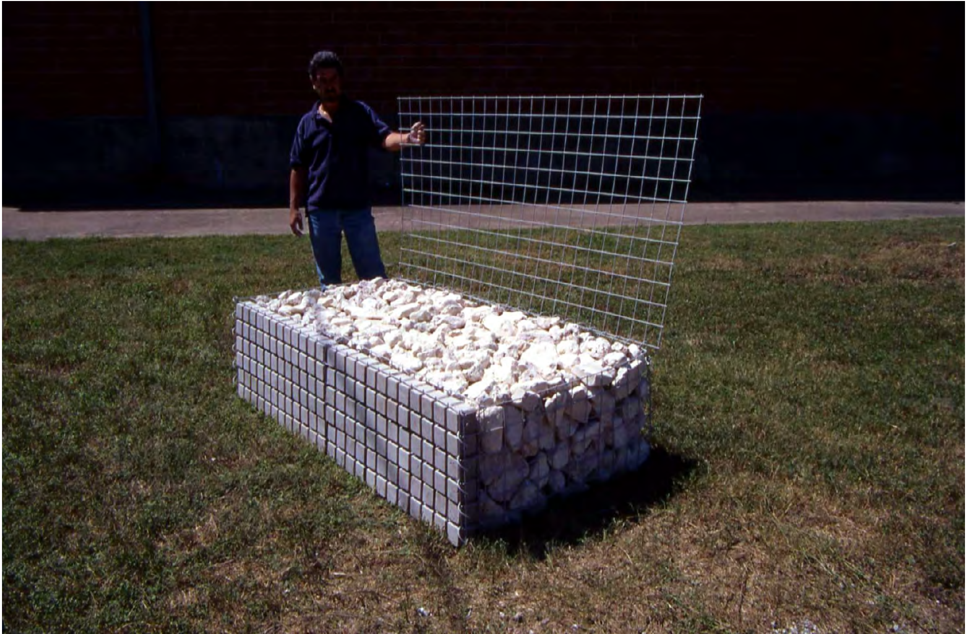
COMPLETED GABION WITH CONCRETE BLOCKS FACING
