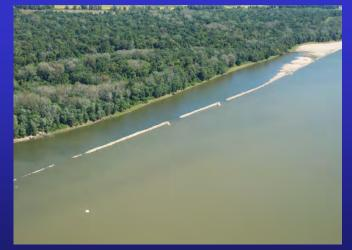
Flow DistributionNotched Off-Bank Revetment— One Corps Serving the Armed Forces and the Nation
