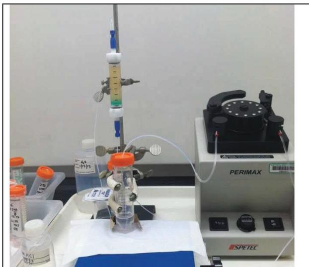
**Figure 2.** Image of cobalt retained on the anion-exchange resin column (bright blue green band at bottom of column) after nickel was eluted.
