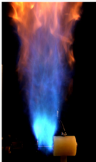
Figure 19: Digital Camera Image of Laser-induced Ignition
