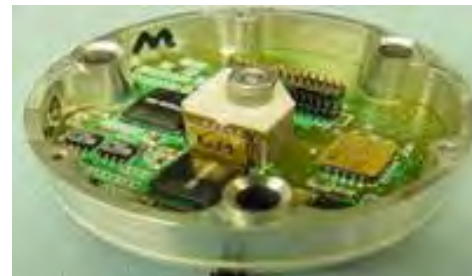
Accel Cluster (shown mounted in vibration isolator)
