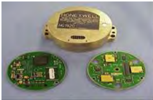
Accel Cluster (shown mounted in vibration isolator)
