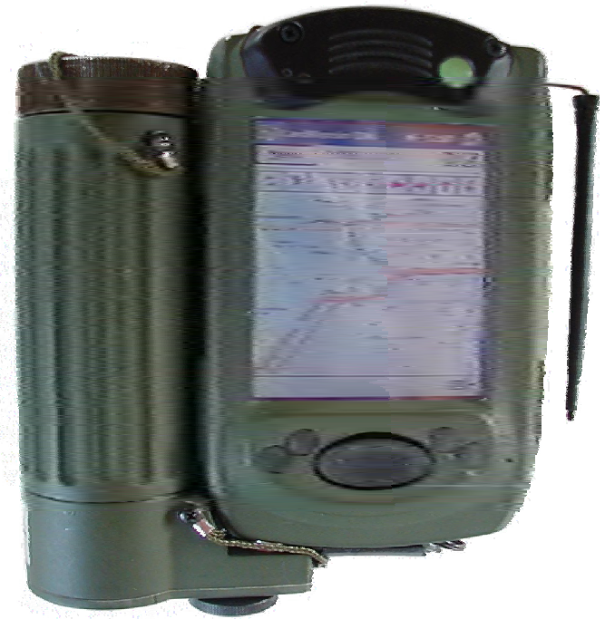
Lightweight Handheld Mortar Ballistic Computer, XM32
