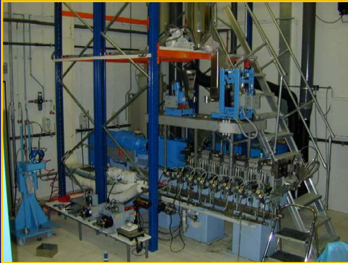
45 mm twin-screw extruder
