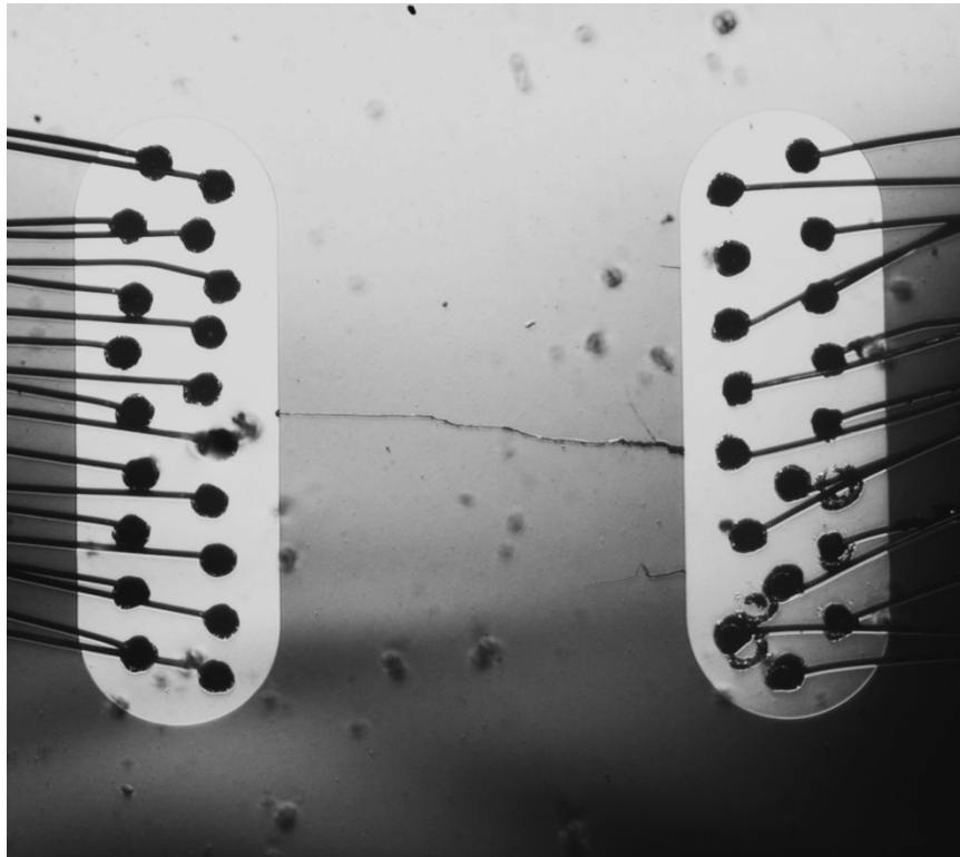
Fig. 1 PCSS device damaged by filaments
