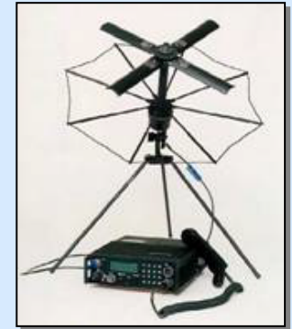
AN/PSC-5 Satellite Radio
