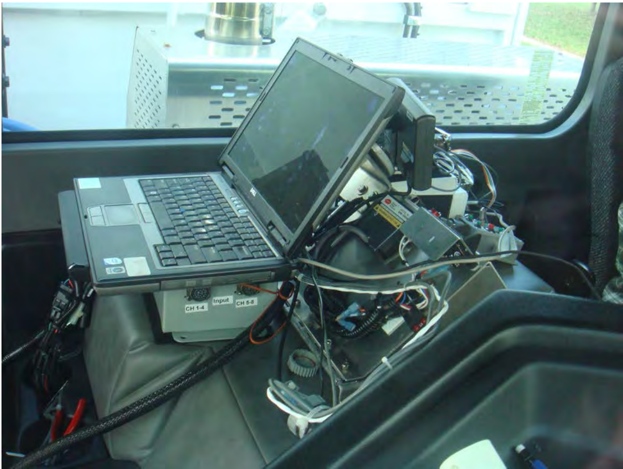
Figure 5-15. On-board Instrumentation for Fuel Economy Data Collection (Photo by Chris Shires, US Army ATC)
