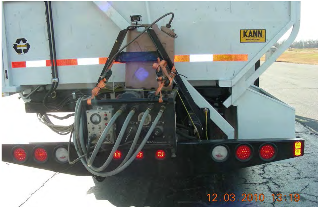
Figure 5-10. Temporary Metering System Used to Capture Fuel Consumption (Photo by Chris Shires, US Army ATC)
