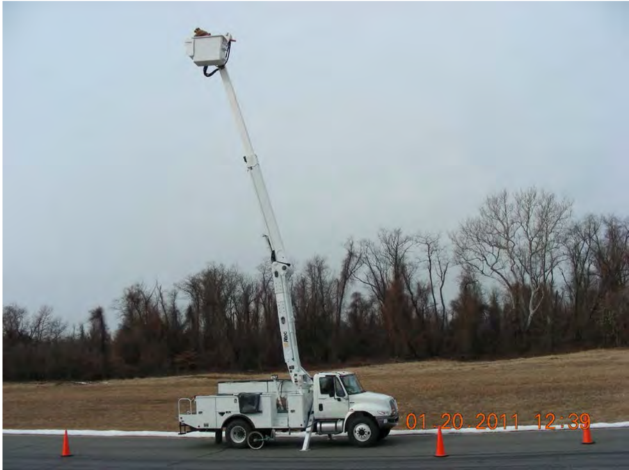
Figure 6-3. Fuel Economy Testing on the Conventional Utility Truck. (Photo by Chris Shires, US Army ATC)
