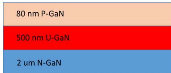
Fig. 3 The GaN wafer profile using the doping profile in Khan et al. 21
