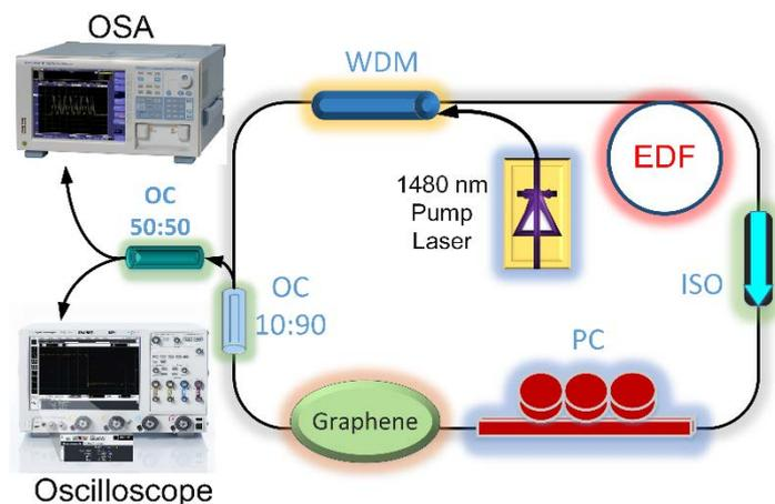
**Figure 1.1** A schematic diagram of the fiber laser setup. SMF: Single-mode fiber, PC: Polarization controller, EDF: Erbium doped fiber, WDM: Wavelength-division multiplexer, OC: Optical coupler, ISO: Isolator, OSA: Optical spectrum analyser.
