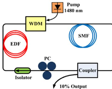
Figure 3.1. A schematic of the Erbium-doped fiber laser. EDF: Erbium-doped fiber. SMF: Single mode fiber. WDM: Wavelength division multiplexer. PC: Polarization controller.
