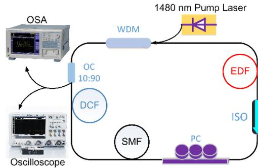
Figure 4.5: A schematic of the Erbium-doped fiber ring laser. EDF: Erbium-doped fiber. SMF: Single mode fiber. DCF: Dispersion compensation fiber. WDM: Wavelength division multiplexer. PC: Polarization controller. ISO: Isolator. OC: Output coupler. OSA: Optical spectrum analyzer.
