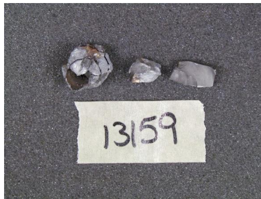
Fig. 13 Residual penetrator from impact versus CoorsTek alumina AD-995
