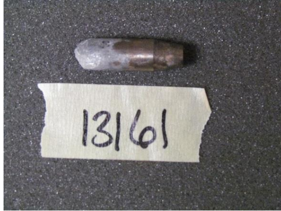
Fig. 14 Residual penetrator from impact versus HEW alumina
