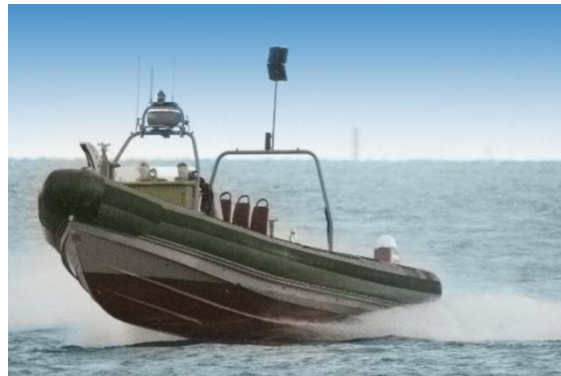
Figure 3. FRISC with fore and aft corner reflectors.
