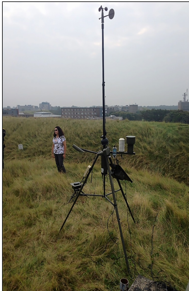
Figure 16. TACMET measuring surface values at the shore station launch.
