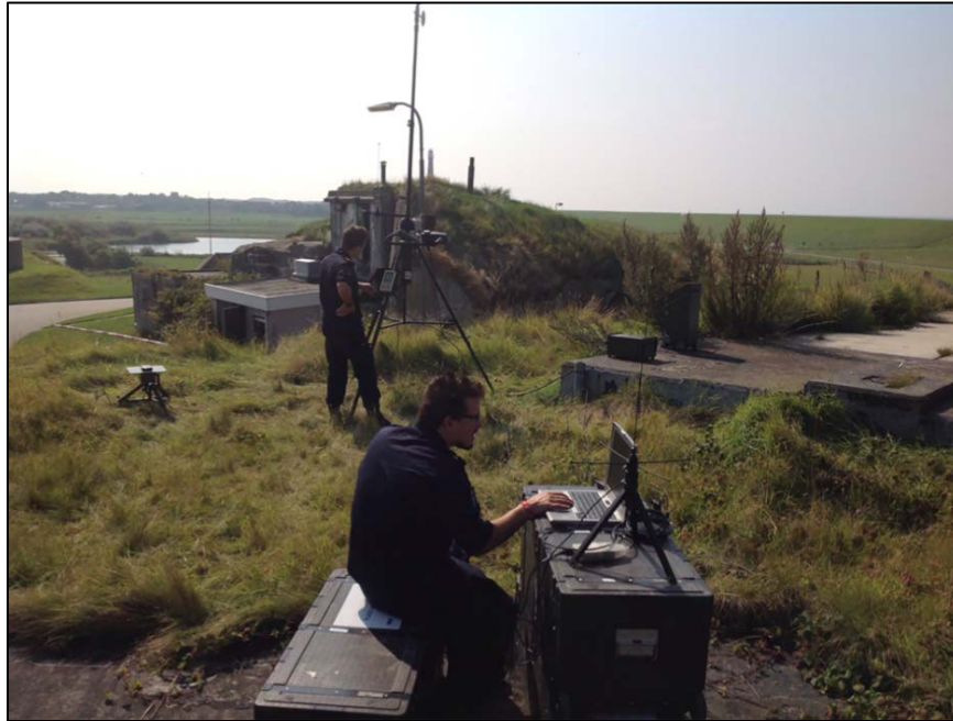
Figure 11. Shore-site TACMET station and radiosonde launch site.
