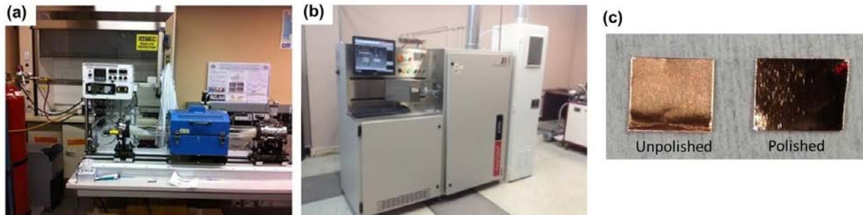
Figure 3.1.1: (a) LPCVD and (b) APCVD systems for graphene growth. (c) Photograph of Cu foils before/after electropolishing.
