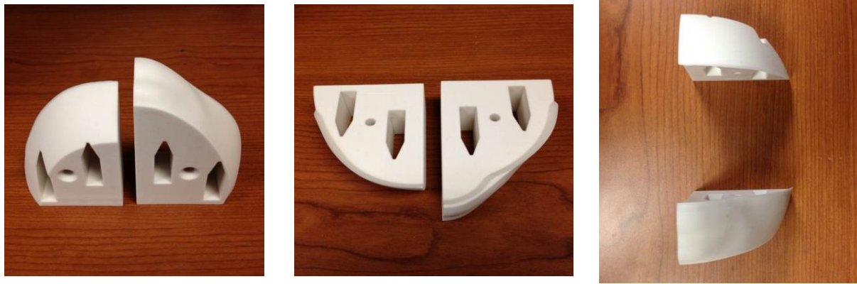
Figure 17: Superior and inferior 3D fixture extension blocks after printing, hand finishing, and sealing. Superior and inferior surfaces (left), internal surfaces (center), anterior surfaces (right).
