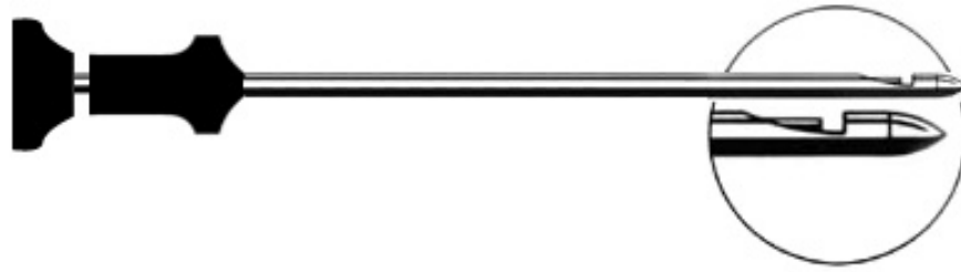
Figure 110: Example of biopsy needle used for disk pressure when combined with a Model 060S pressure sensor.
