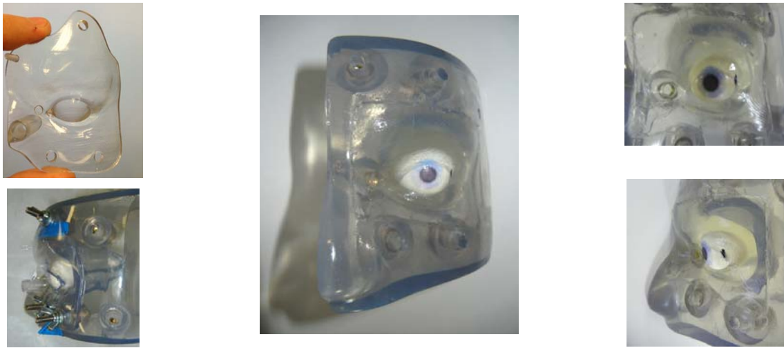
Figure 15: (Left, top) Open eyelid mold. (Left, bottom) Open eyelid mold bolted to 3D orbit. (Middle, Right) 3D printed orbit with 10% gelatin solution to simulate skin, fat, and musculature
