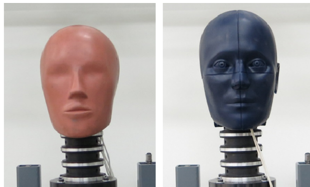
Figure 63: The most commonly used headforms in helmet impact testing, (a) a 50 th percentile male Hybrid III headform and (b) a medium NOCSAE headform, both mounted on a 50 th percentile male Hybrid III neck.
