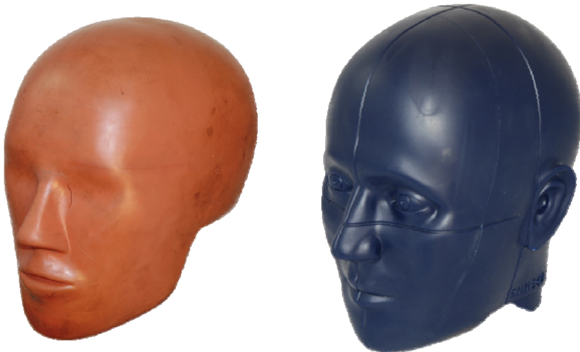
Figure 56: The Hybrid III (left) and NOCSAE (right) headforms are the most commonly used headforms in helmet impact performance testing.
