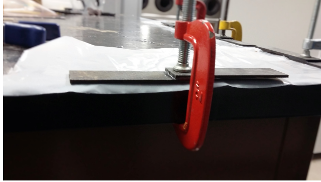
Figure 3.2: C-clamps were used for applying constant pressure.
