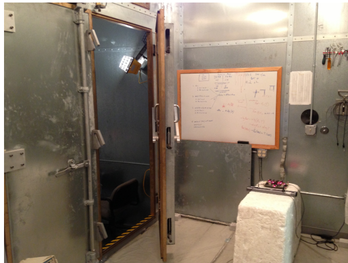
Figure 4.14: Position of the shielded door between the main chamber and the ante chamber for High Coupling configuration.
