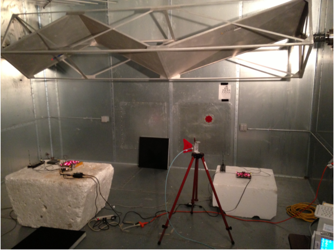
Figure 2.2: Main chamber of the coupled reverberation chambers of the NSWCCD. This picture was taken from the doorway connecting the main chamber to the ante chamber. The horizontal Z-fold mechanical tuner along the north wall is shown at the top of the image. One of the horn antennas used for the impulse measurements is on the tripod in the middle of the image. Two of the wireless nodes (described in Chapter 3) are shown on non-absorbing Styrofoam blocks.
