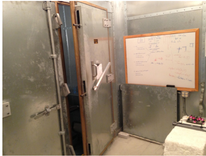
Figure 4.13: Position of the shielded door between the main chamber and the ante chamber for Medium Coupling configuration.
