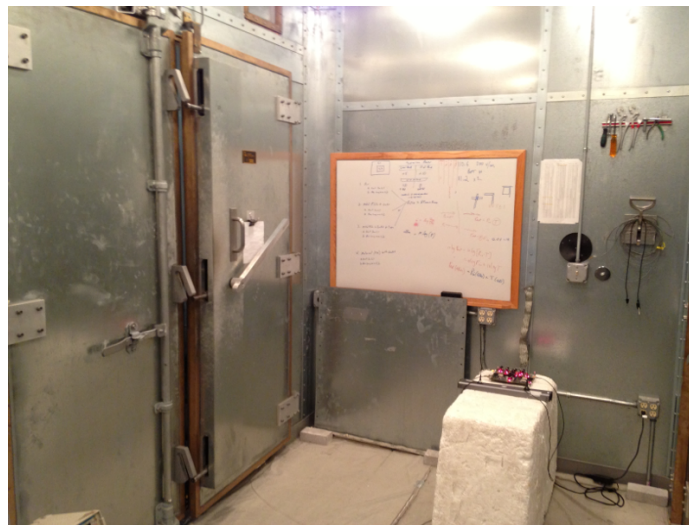
Figure 4.12: Position of the shielded door between the main chamber and the ante chamber for Low Coupling configuration.
