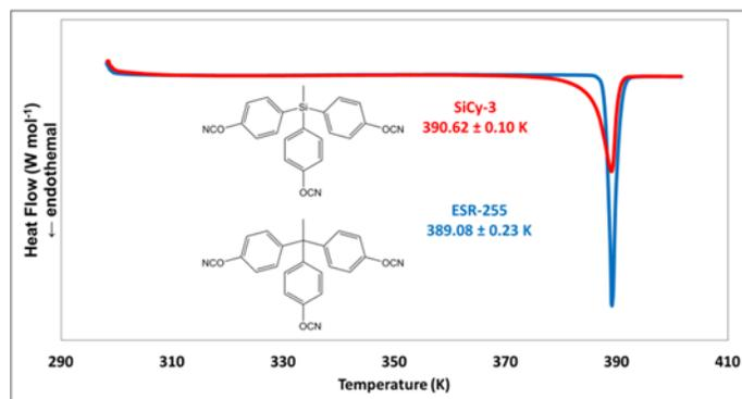
The DSC plots for the cyanate ester monomer, ESR-255, and its silicon counterpart, SiCy-3. Although structurally different, they are quite thermodynamically similar.
