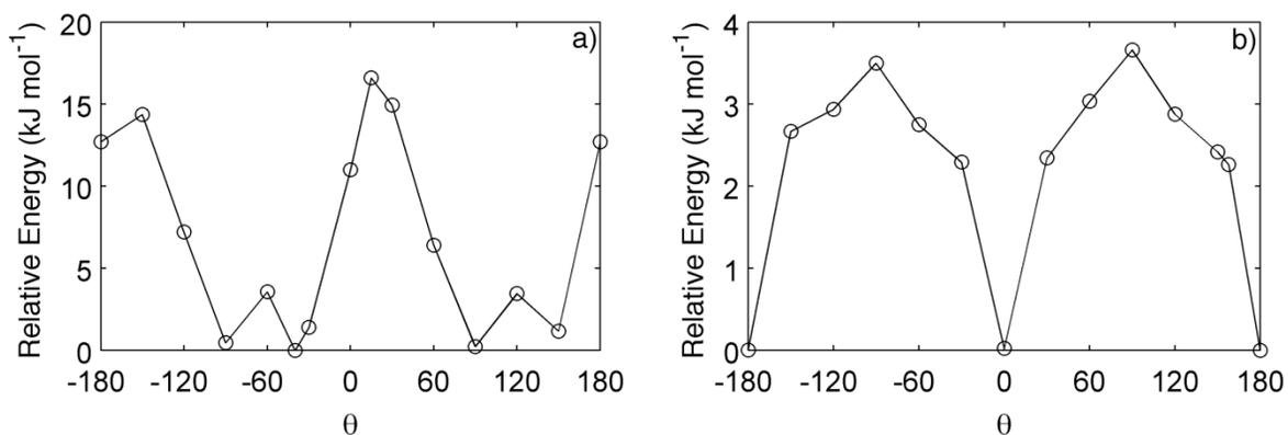
**Figure 10.** Relative Energy for a) BADCy and b) SiMCy as function of the dihedral angle  $\theta$ .
