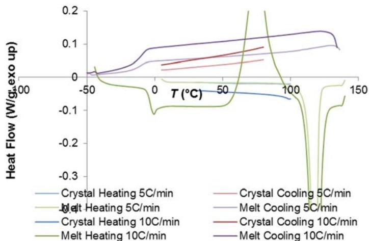
Figure S1-5. Raw DSC data for SiCy-3 sample #1. Note that during the “melt heating” segment, the sample is actually crystalline at the slower heating rate, and that it re-crystallizes at the faster heating rate.
