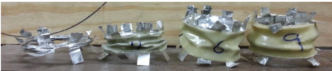
Figure 21: Front view of crushed cylinders increasing in polyurea mass from left to right
