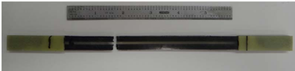
Figure 6. Continuous Carbon Fiber Composite Specimen After Testing
