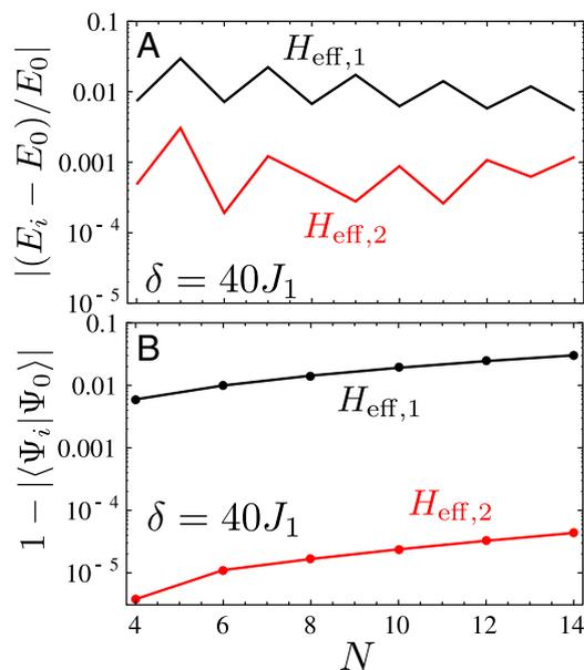
**Fig. 9.** (A) Comparison of ground-state energy error  $|(E_i - E_0)/E_0|$  and (B) ground-state overlap  $|\langle \Psi_0 | \Psi_i \rangle|$  as a function of  $N$  for Hamiltonians  $H_{\text{eff},1}$  (black) and  $H_{\text{eff},2}$  (red) with detuning  $\delta/J_1 = 40$ .
