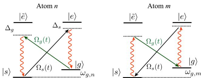
**Fig. 3.** Atomic “butterfly” level structure. Two pump fields  $\Omega_s$  and  $\Omega_g$ , tuned to couple to the same GM photon, are introduced to control  $XX$  and  $YY$  interactions independently.
