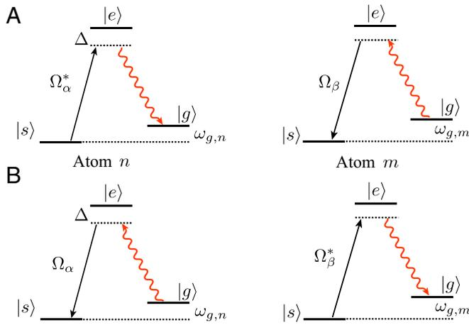
**Fig. 2.** Schematics to engineer long-range spin exchange interactions via resonant Raman-scattering processes. Spin exchanges (A)  $|s_n, g_m\rangle \rightarrow |g_n, s_m\rangle$  and (B)  $|g_n, s_m\rangle \rightarrow |s_n, g_m\rangle$  are allowed only when the condition  $\omega_{g,m} - \omega_{g,n} = \tilde{\omega}_\beta - \tilde{\omega}_\alpha$  is satisfied.  $\Omega_\alpha/\Delta$  and  $\Omega_\beta/\Delta$  control the exchange rate.
