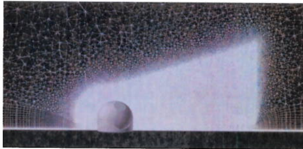
Figure 8. Two dimensional view of the hybrid mesh around the turret.
