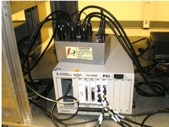
**Fig. 6** Power supply with 6 feeds, on top of PXi chassis with 6 serial port output
