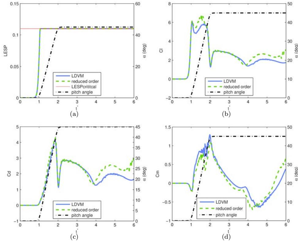
Figure 6.5: Case 3: Comparison of predictions of the reduced order method and LDVM. Variation with  $t^* = tU/c$  of: (a) LESP, (b) lift coefficient, (c) drag coefficient, and (d) pitching moment coefficient about the quarter chord.
