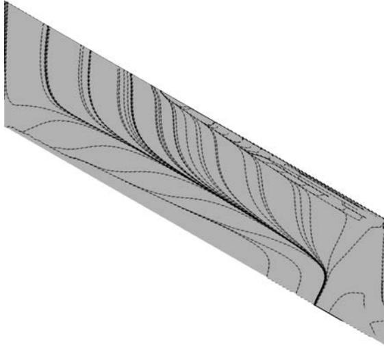
(a) Upper-surface skin-friction lines for case 10,  $t^* = 1.080$ ,  $\alpha = 2.79$  deg.
