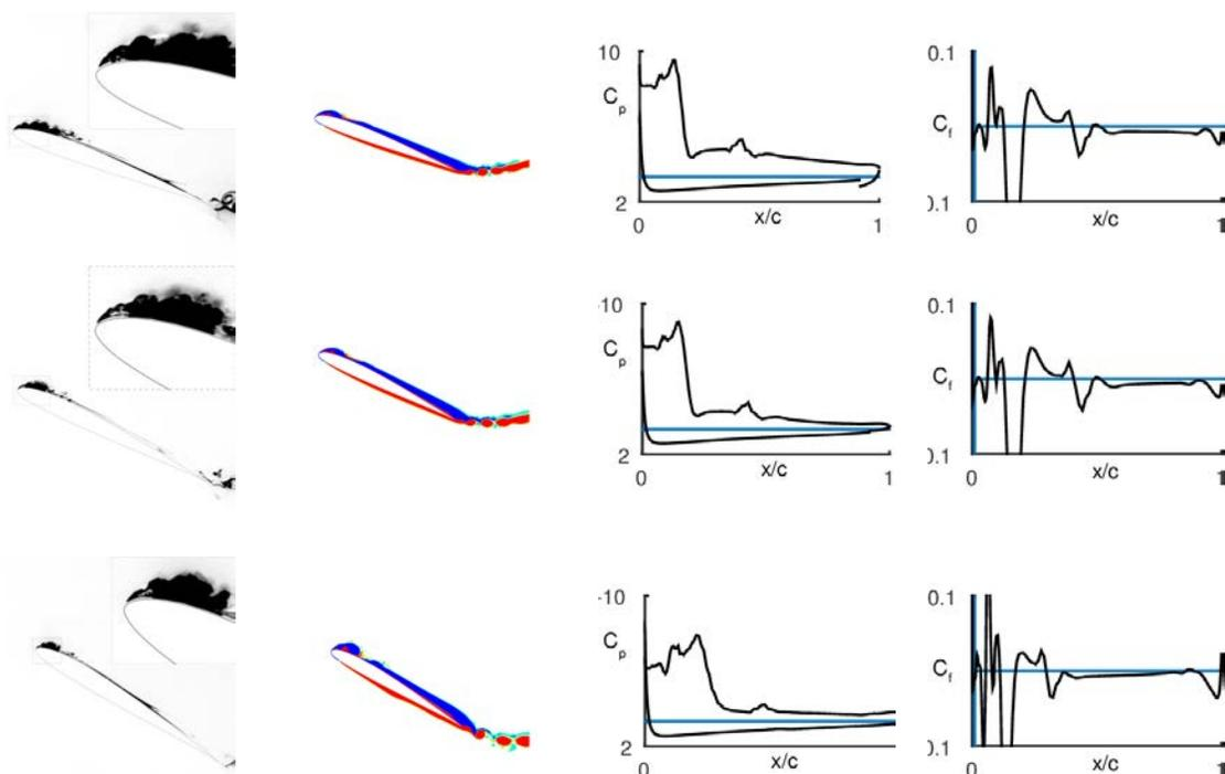
Figure 5.7: Case study 1: left to right - flow visualization from experiment, vorticity plots from CFD,  $C_p$  (upper and lower surfaces) and  $C_f$  (upper surface) distributions from CFD at  $\Delta LES P = 0.1$  after the instants of LEV initiation. Top to bottom - pivot location at leading edge, quarter chord and three-quarter chord.
