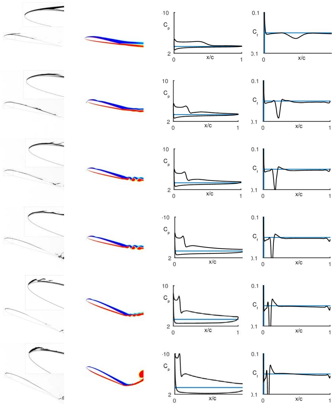
Figure 5.10: Case study 2: left to right - flow visualization from experiment, vorticity plots from CFD,  $C_p$  (upper and lower surfaces) and  $C_f$  (upper surface) distributions from CFD at the instants of LEV initiation. Top to bottom - pitch rate of 0.01, 0.03, 0.05, 0.1, 0.2 and 0.4).
