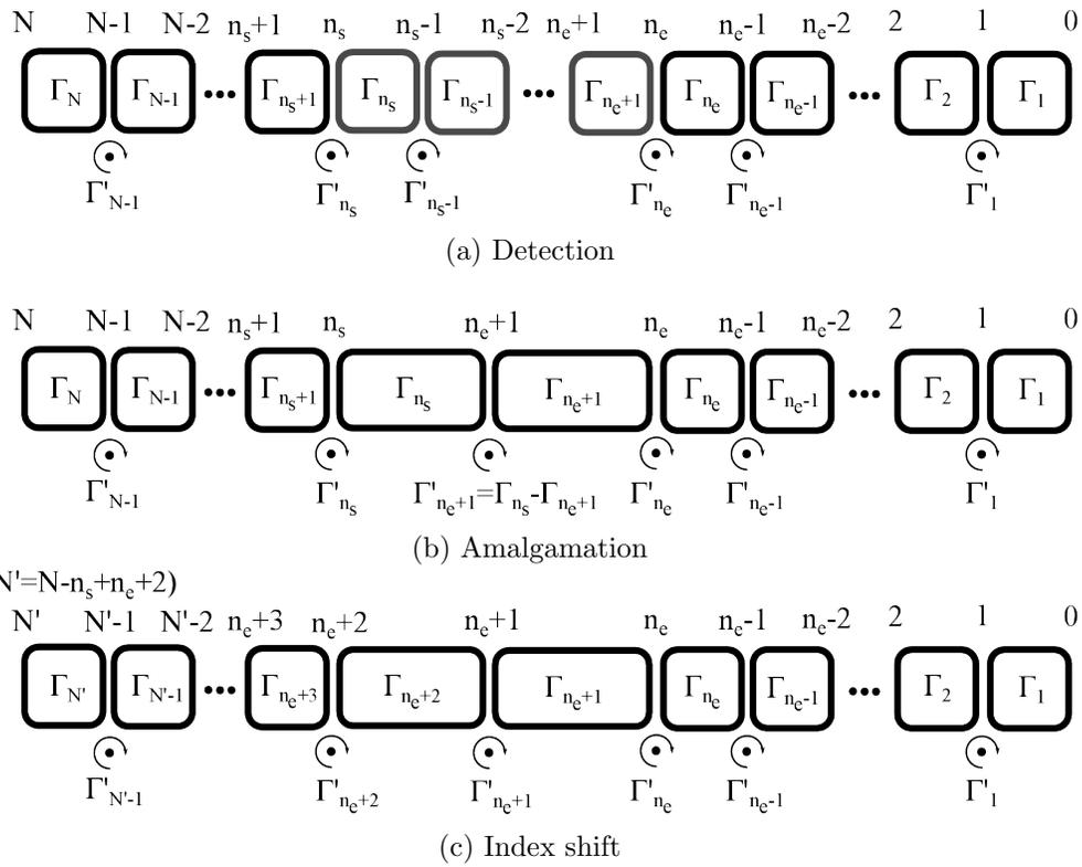
Figure 7.11: Schematic description of procedure of amalgamation.
