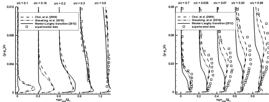
Figure 3.11: Profile of the rms streamwise velocity fluctuations obtained by a hybrid LES/RANS computation; individual profiles are separated by a horizontal profile of 0.3 (left) and 0.2 (right).
