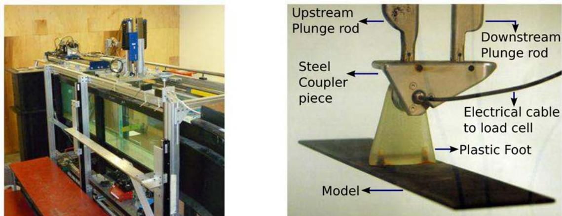
Figure 4.1: Test section and portion of motion rig mounted above test section of the AFRL Horizontal Free-surface Water Tunnel (left).  $c = 3$ " flat plate with force balance mounted between steel coupler piece and plastic foot connecting to the plate (right). Dye injection is from a 0.5 mm diameter slot at the plate leading and trailing edges,  $\frac{3}{4}$  spanwise location.
