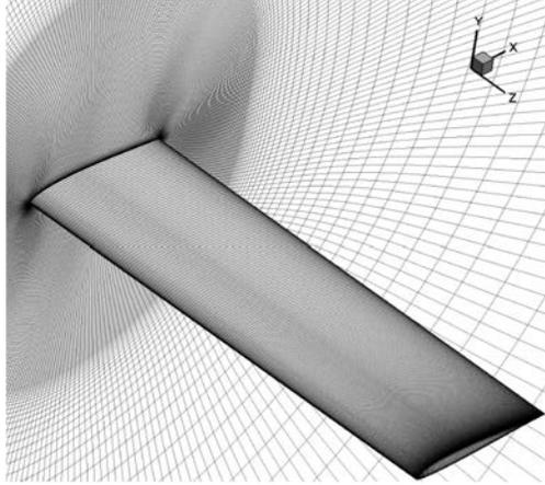
Figure 3.4: Representative mesh distribution for CFD analysis.
