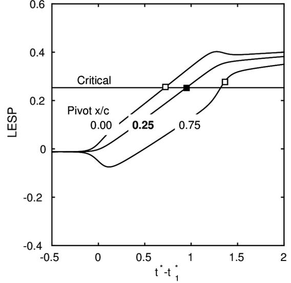
Figure 5.5: Case study 1: LESP variation with time, and LESP values at which LEV formation is initiated (kinematics with different pivot locations).
