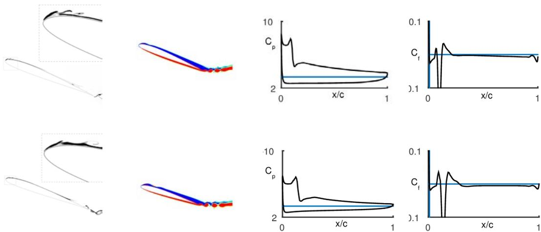
Figure 5.18: Flow visualization from experiment, vorticity plots from CFD,  $C_p$  (upper and lower surfaces) and  $C_f$  (upper surface) distributions from CFD at the instant of LEV initiation for cases 1 and 15.
