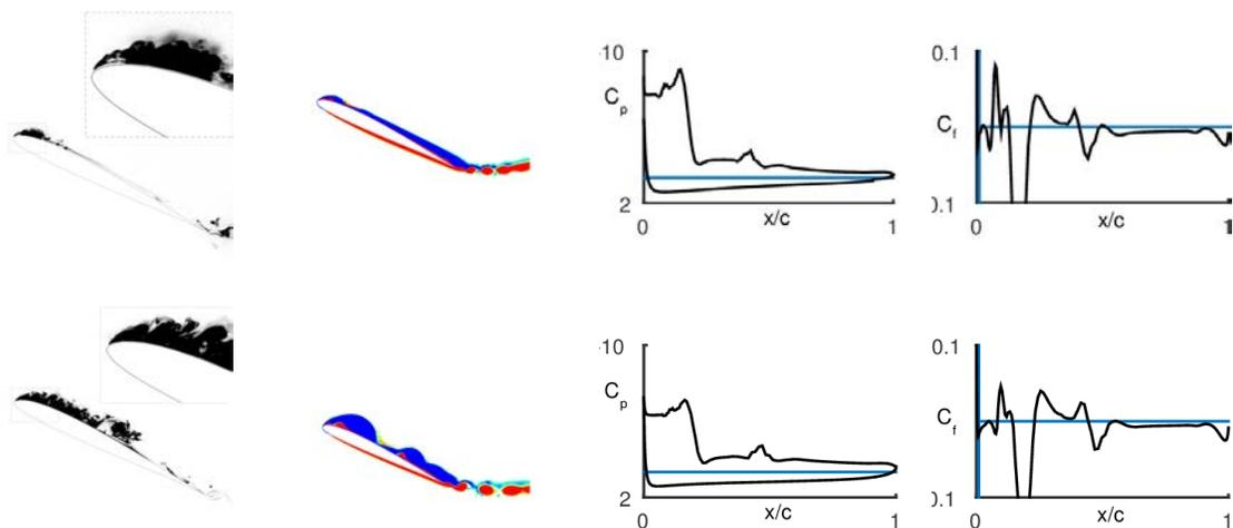
Figure 5.19: Flow visualization from experiment, vorticity plots from CFD,  $C_p$  (upper and lower surfaces) and  $C_f$  (upper surface) distributions from CFD at some  $\Delta LESP$  after the initiation of LEV formation for cases 1 and 15.
