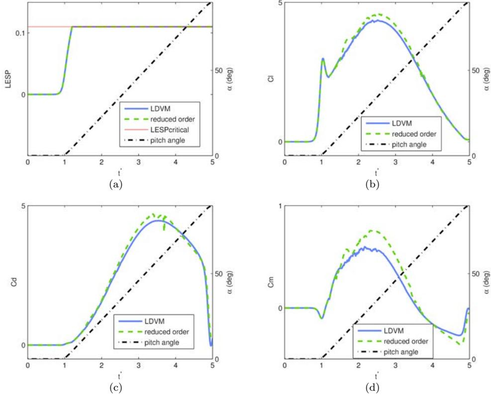
Figure 6.1: Case 1: Comparison of predictions of the reduced order method and LDVM. Variation with  $t^* = tU/c$  of: (a) LESP, (b) lift coefficient, (c) drag coefficient, and (d) pitching moment coefficient about the mid chord.
