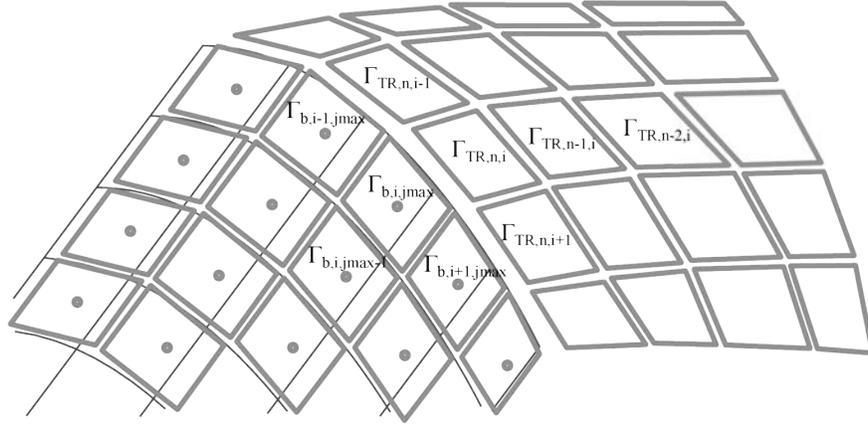
Figure 7.3: Schematic description of separated tip flow model.
