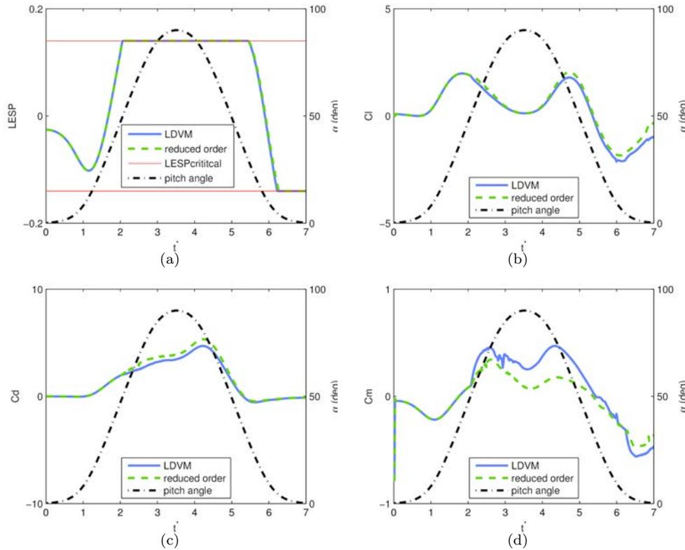
Figure 6.3: Case 2: Comparison of predictions of the reduced order method and LDVM. Variation with  $t^* = tU/c$  of: (a) LESP, (b) lift coefficient, (c) drag coefficient, and (d) pitching moment coefficient about the quarter chord.
