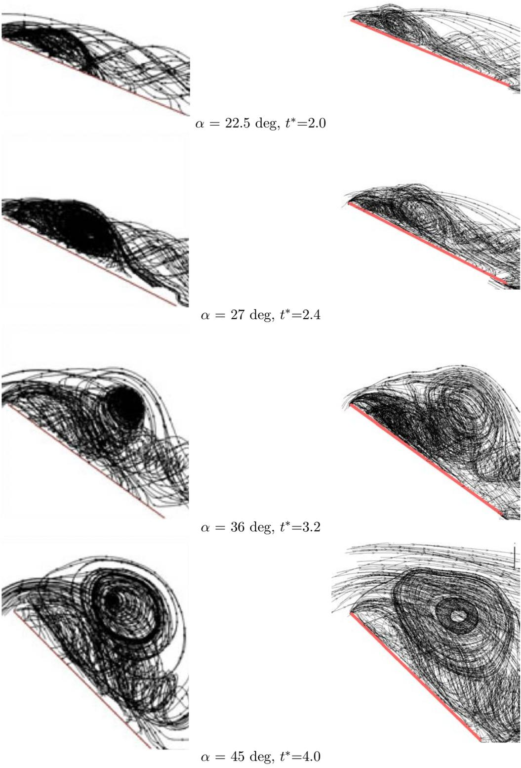
Figure 3.6: Side views of three-dimensional streamline patterns as a function of angle of attack. Left: PIV experiment. Right: CFD simulation.
