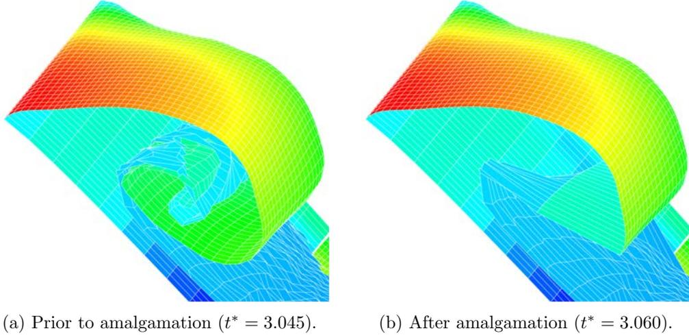
Figure 9.10: Snapshots of three-dimensional amalgamation method
