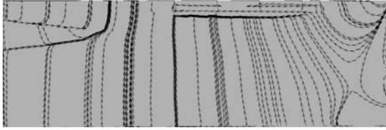
(a) Upper-surface skin-friction lines for case 6,  $t^* = 1.575$ ,  $\alpha = 19.75$  deg.
