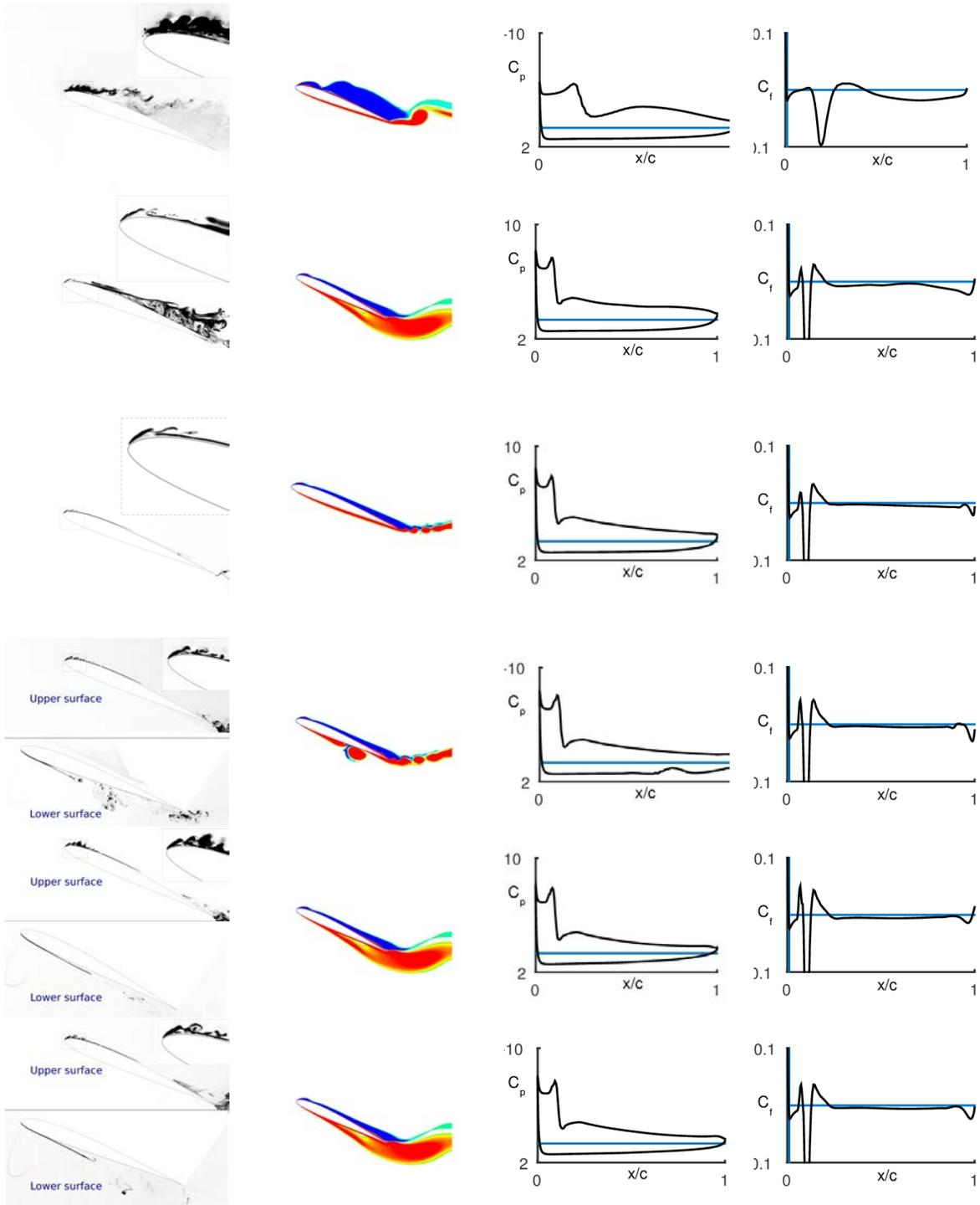
Figure 5.14: Case study 3: left to right - flow visualization from experiment, vorticity plots from CFD,  $C_p$  (upper and lower surfaces) and  $C_f$  (upper surface) distributions from CFD at the instants of LEV initiation. Top to bottom - starting pitch angles of 10, 5, 0, -5, -10 and -15 deg).
