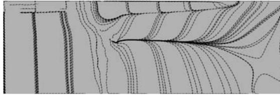
(a) Upper-surface skin-friction lines for case 12,  $t^* = 1.605$ ,  $\alpha = 20.80$  deg.
