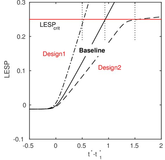
Figure 5.23: LESP variation with time for the baseline case and the two design cases. As required by the design criteria, the intersection of instantaneous  $LESP$  with critical  $LESP$  is at  $t^* - t_1^* = 0.5$  and  $1.5$  respectively.
