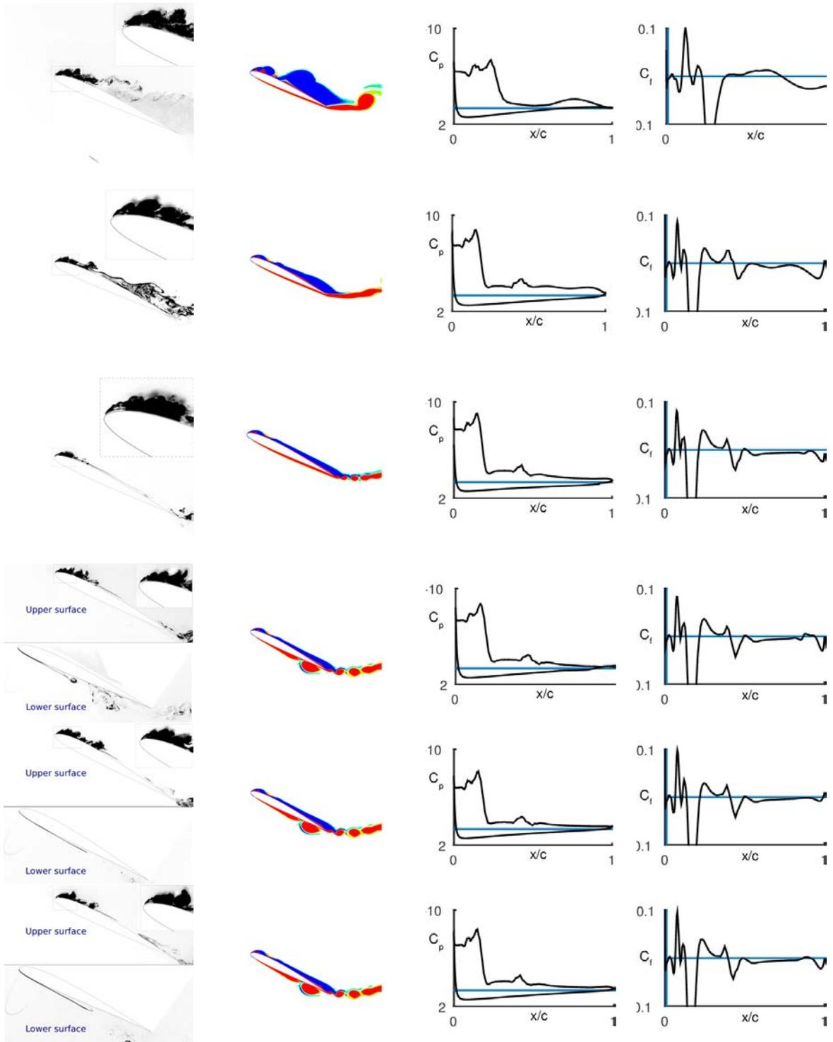
Figure 5.15: Case study 3: left to right - flow visualization from experiment, vorticity plots from CFD,  $C_p$  (upper and lower surfaces) and  $C_f$  (upper surface) distributions from CFD at  $\Delta LES P = 0.1$  after the instants of LEV initiation. Top to bottom - starting pitch angles of 10, 5, 0, -5, -10 and -15 deg).
