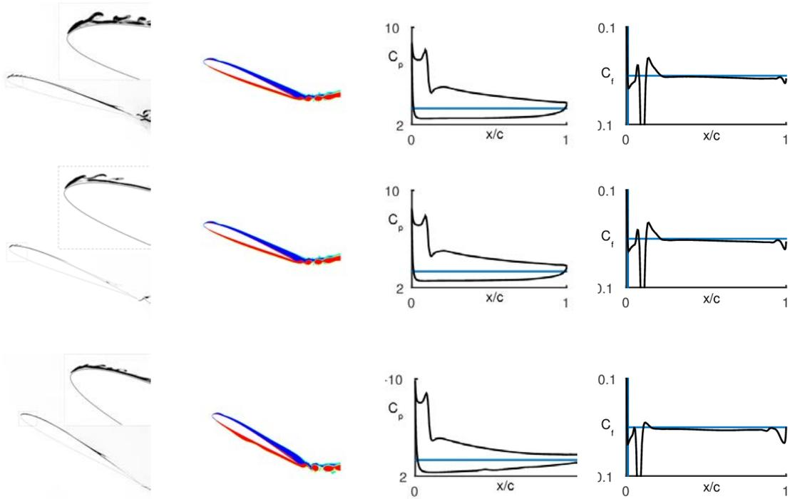
Figure 5.6: Case study 1: left to right - flow visualization from experiment, vorticity plots from CFD,  $C_p$  (upper and lower surfaces) and  $C_f$  (upper surface) distributions from CFD at the instants of LEV initiation. Top to bottom - pivot location at leading edge, quarter chord and three-quarter chord.
