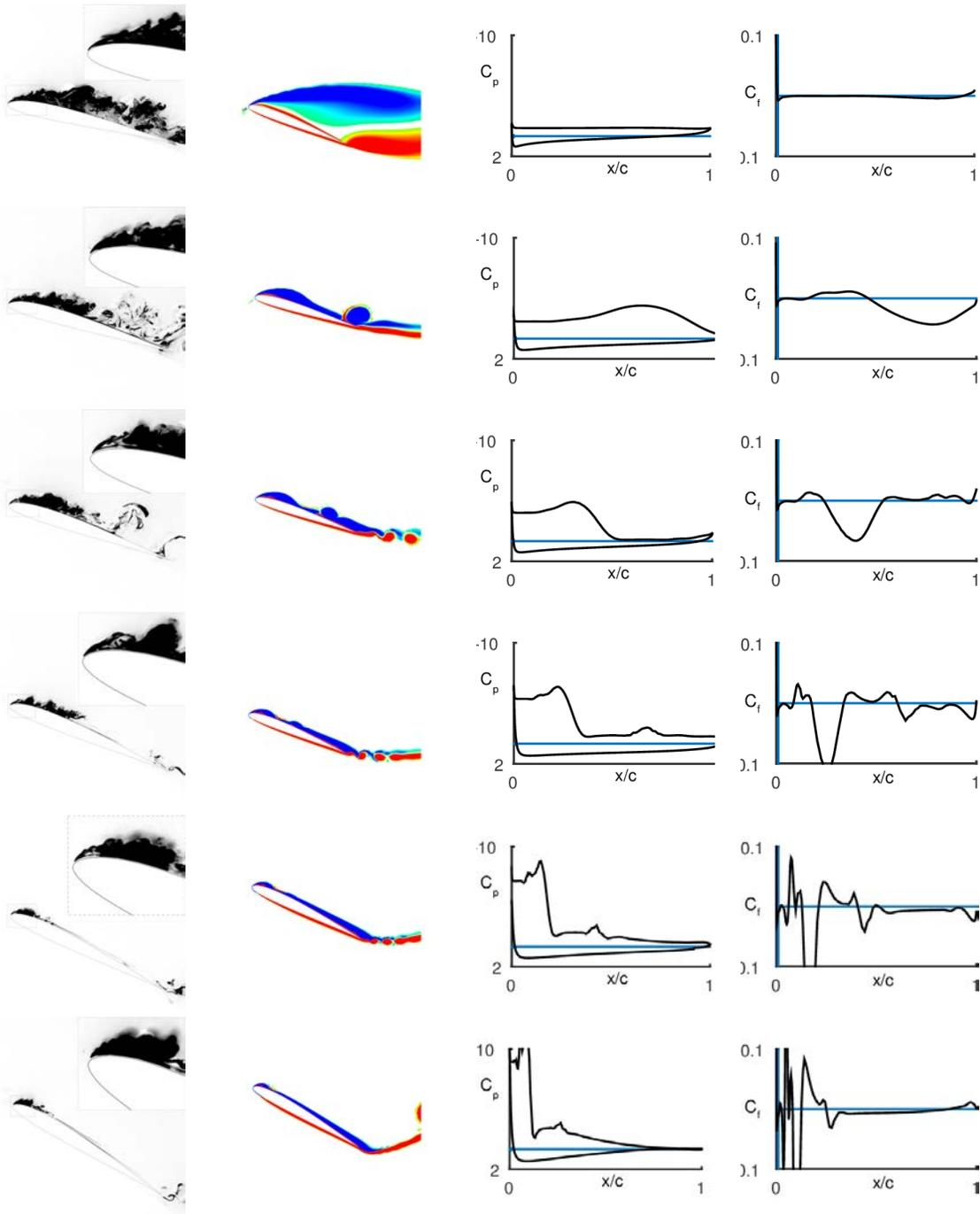
Figure 5.11: Case study 2: left to right - flow visualization from experiment, vorticity plots from CFD,  $C_p$  (upper and lower surfaces) and  $C_f$  (upper surface) distributions from CFD at  $\Delta LES P = 0.1$  after the instants of LEV initiation. Top to bottom - pitch rate of 0.01, 0.03, 0.05, 0.1, 0.2 and 0.4).
