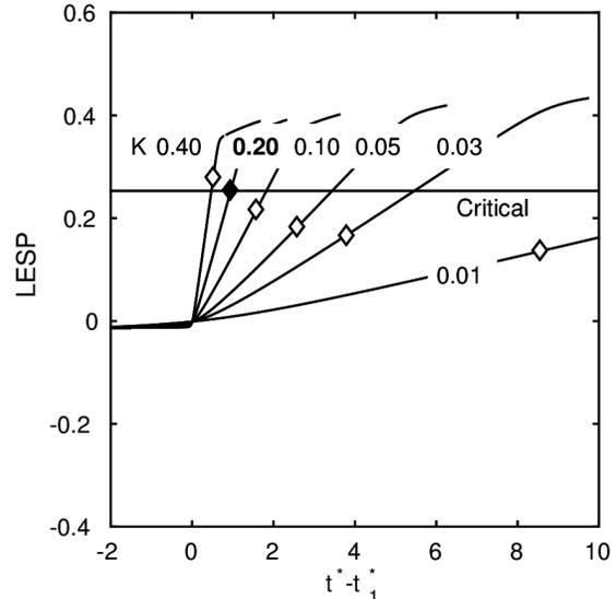
Figure 5.9: Case study 2: LEVP variation with time, and LEVP values at which LEV formation is initiated (kinematics with different pitch-rates).
