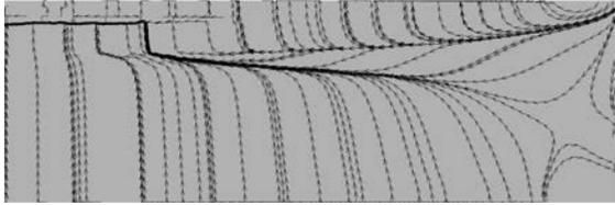
(a) Upper-surface skin-friction lines for case 1,  $t^* = 1.710$ ,  $\alpha = 24.41$  deg.
