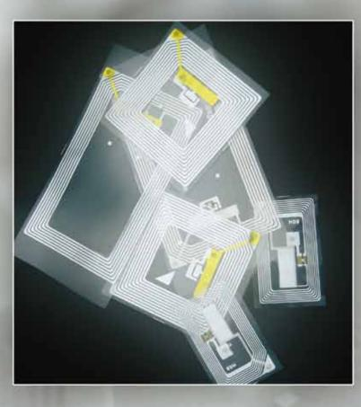
ost radio frequency identification (RFID) tags contain at least two parts. One is an integrated circuit for storing and processing information, modulating and demodulating a radio frequency signal, and other specialized functions. The second is an antenna for receiving and transmitting the signal.
