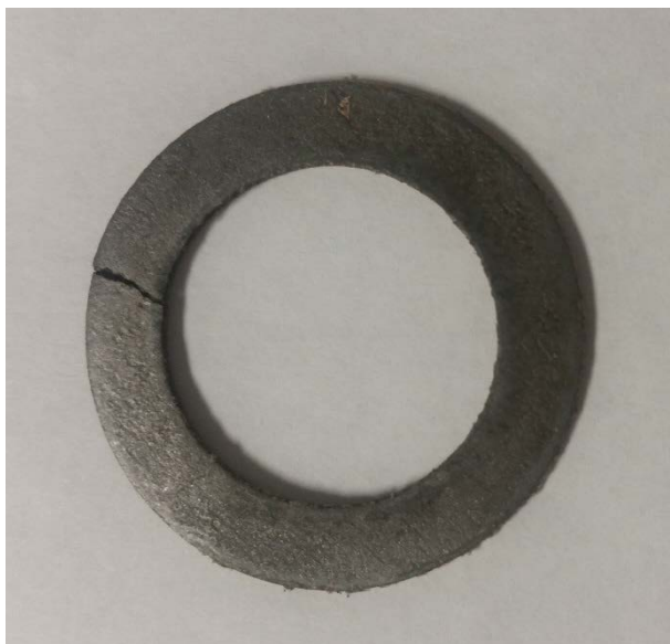
Figure 1. Damaged combustion chamber gasket caused by over pressurization while testing ATJ samples.
