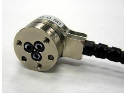
Figure 5.1 ATI Nano-17 miniature six-component balance
