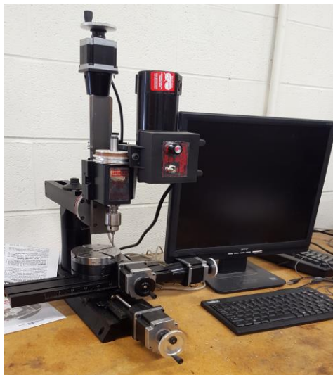
Fig. 13.1 Sherline milling machine with control computer
