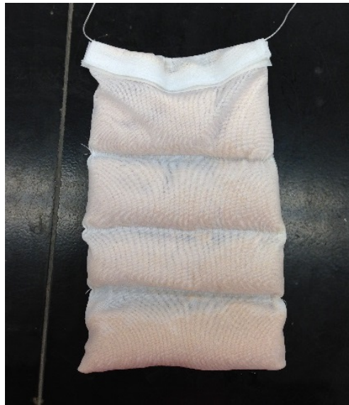
Figure 34. One of three mesh bags that were deployed into the continuous AnMBR system containing approximately 370 g of Purolite® Tanex each.
