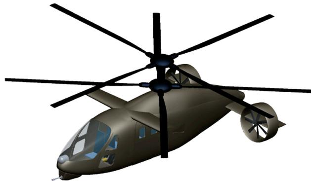
Figure 1. Coaxial Compound Helicopter (CCH) configuration.
