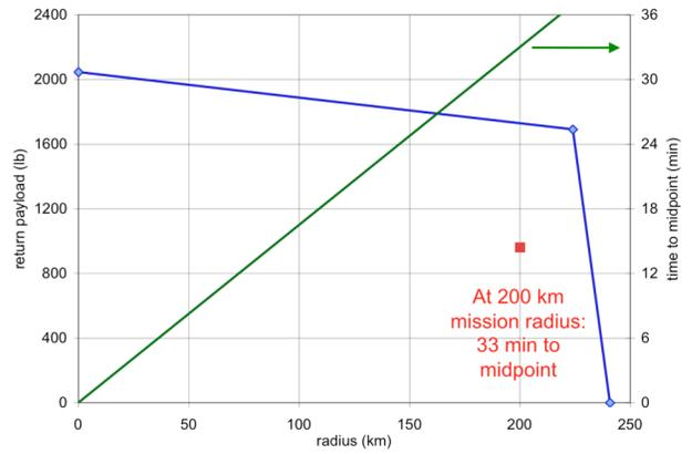
Figure 26. MEDEVAC payload-radius.
