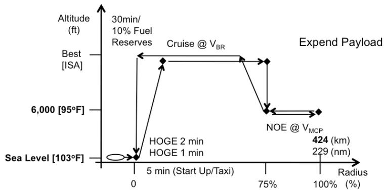
Figure 21. Counter-IADS UAS mission profile. Payload 1600 lb.
