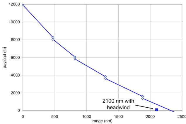
Figure 27. Self-deploy payload-range; takeoff weight 18200 lb (1.9 SDGW).
