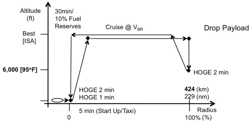
Figure 17. Cargo UAS mission profile. Payload 1200 lb.
