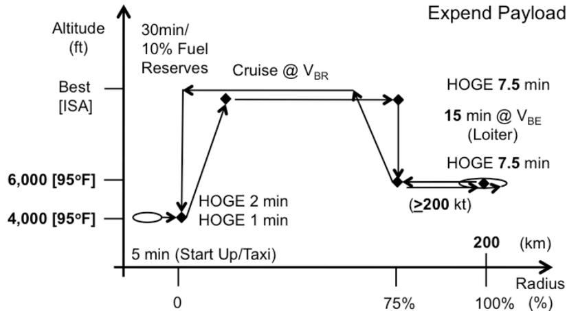
Figure 14. Light attack mission profile. Payload 1020 lb.
