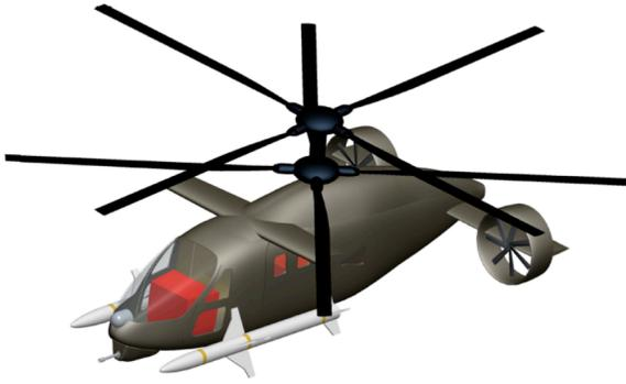
Figure 22. Counter-IADS UAS configuration.
