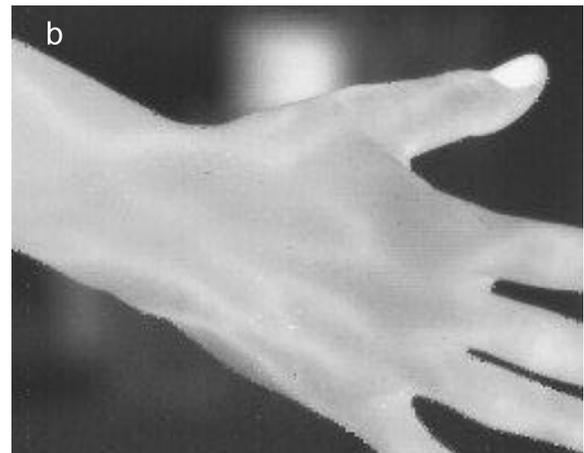
**Fig. 3.** (a) Zero-bias response spectra of 5-stage mid-IR interband cascade photo-detector at several operating temperatures. The atmospheric CO<sub>2</sub> absorption at 4.2 μm and water absorption lines around 2.7 μm are clearly seen. (b) Thermal image acquired by the  $320 \times 256$  IC FPA operating at 80 K.
