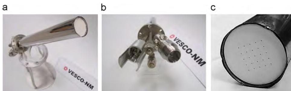
Fig. 1. (a) Custom NbCl<sub>5</sub> cell with (b) tip filament, bulk water, tip and bulk thermocouple feedthroughs, and (c) a 5 × 5 hole pattern aperture plate.
