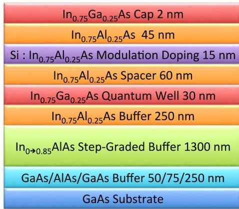
Fig. 1. Schematic layer structure of  $\text{In}_{0.75}\text{Ga}_{0.25}\text{As}/\text{In}_{0.75}\text{Al}_{0.25}\text{As}$  quantum wells.
