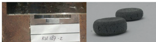
Figure 7. Left: RU187 cylindrical sample and retaining ring attached with double-sided tape to drop weight (top). Right: permanent deformation of the samples after drop weight impact.
