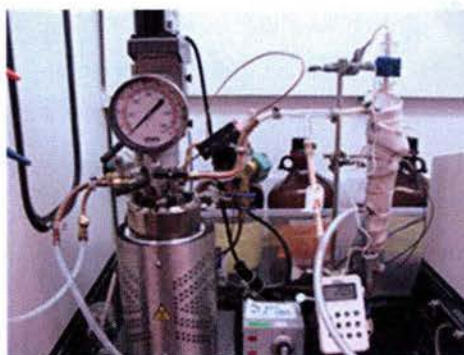
Fig 2.5.2. Laboratory setup of the dual reactor system
