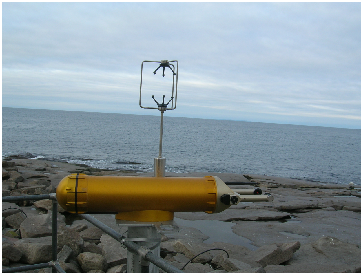
FIG. 2. The cloud imaging probe from Droplet Measurement Technologies and the Gill sonic anemometer/thermometer mounted on the foghorn platform on Mt. Desert Rock.
