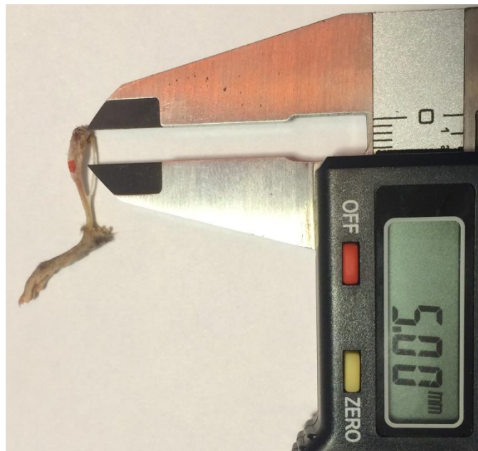
Fig. 20: Strain gauges were positioned on the anteromedial surface of the tibia approximately 5 mm distal to the tibial plateau.
