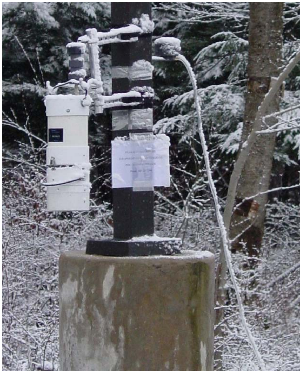
Figure 3-2. MiniVol™ (Left) and Deployable Particulate Sampler (Right) operating at Fort Drum, New York, November, 2006.
