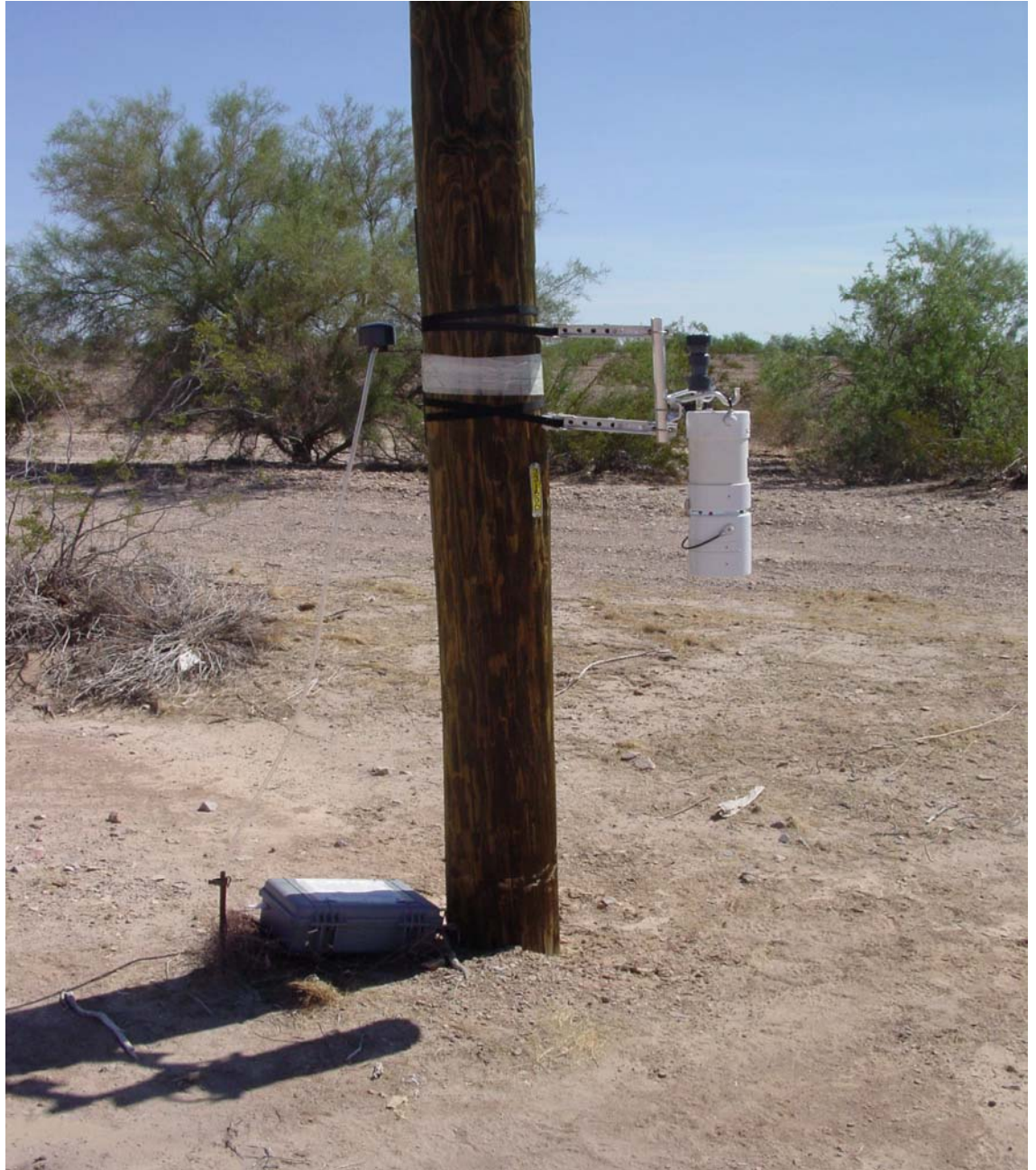
Figure 3-1. Deployable Particulate Sampler (Left) and MiniVol TM (Right) operating at Yuma Proving Grounds, Arizona, September, 2006.
