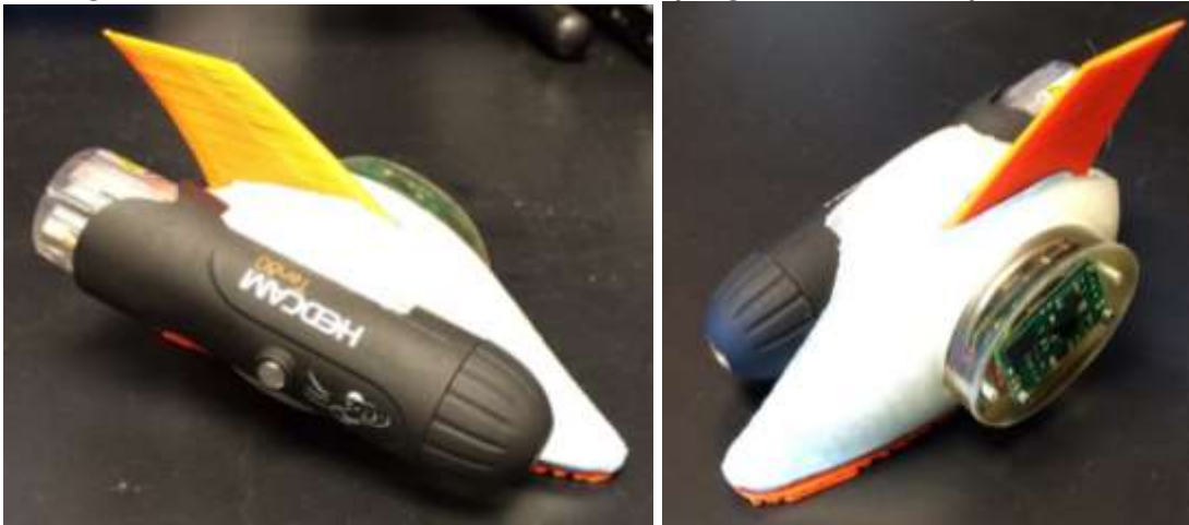
Figure 6. Camera&accelerometer version of tag attached to the fin model.
