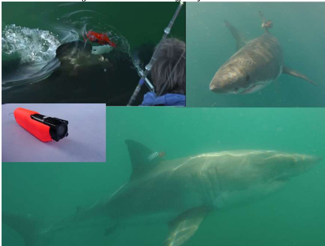
Figure 1. Panels illustrate attachment of shark CATS data logger and camera, accelerometer tag to a mature white shark off California.
