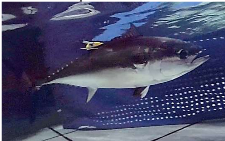
Figure 7. Symmetrical (two accelerometers) version of tag attached on BFT in T2 tank in Hopkins Marine Station.
