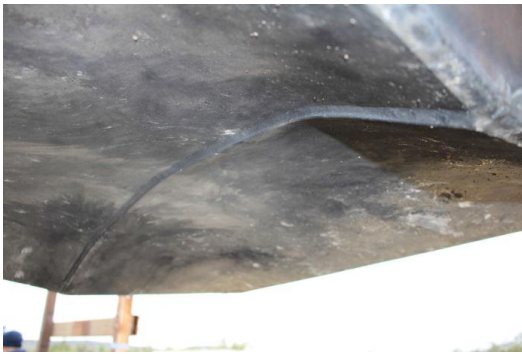
Fig. 14 Blast box V-hull permanent deformation shown in bottom view
