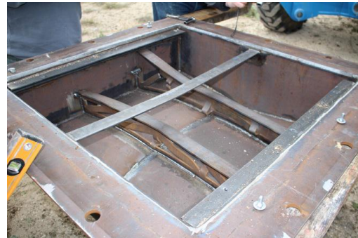
Fig. 13 The deformation of the V-Hull after the live fire test shown in top view
