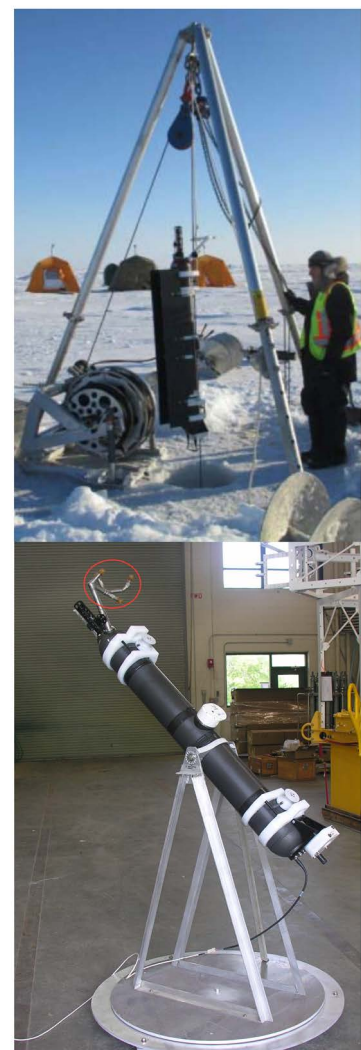
Figure 3. Right. Photograph of an MIZ ITP-V being deployed (top) and in a test jig used to validate sensor orientations (bottom).
