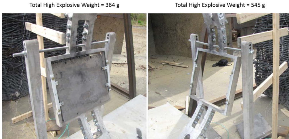
Fig. 5 The detectors and shear tabs following experiments in which 364 g and 545 g of Detasheet C were detonated at the center of the MEFCT support structure
