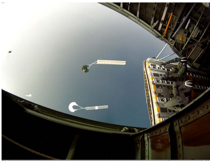
Figure 2. AXCTD (gray) and AXCP (white) being hand-launched simultaneously from rear ramp of USCG C-130H during August 2013 SIZRS flight.
