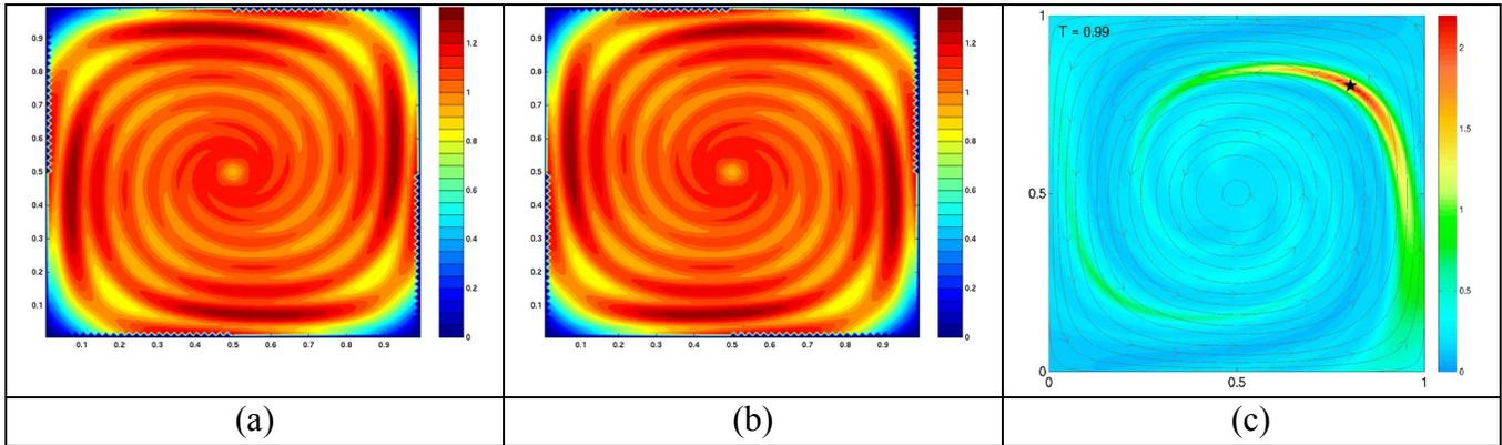
**Figure 1: Comparing LCS to mutual information for reversible swirl flow: (a) forward FTLE (b) backward FTLE (c) mutual information integrated starting from a point in the lower right of the domain to the present time. The mutual information field is correlated with the attractors of the backward FTLE (b), as shown by the mutual information contours spiraling in the same sense as the backward FTLE.**
