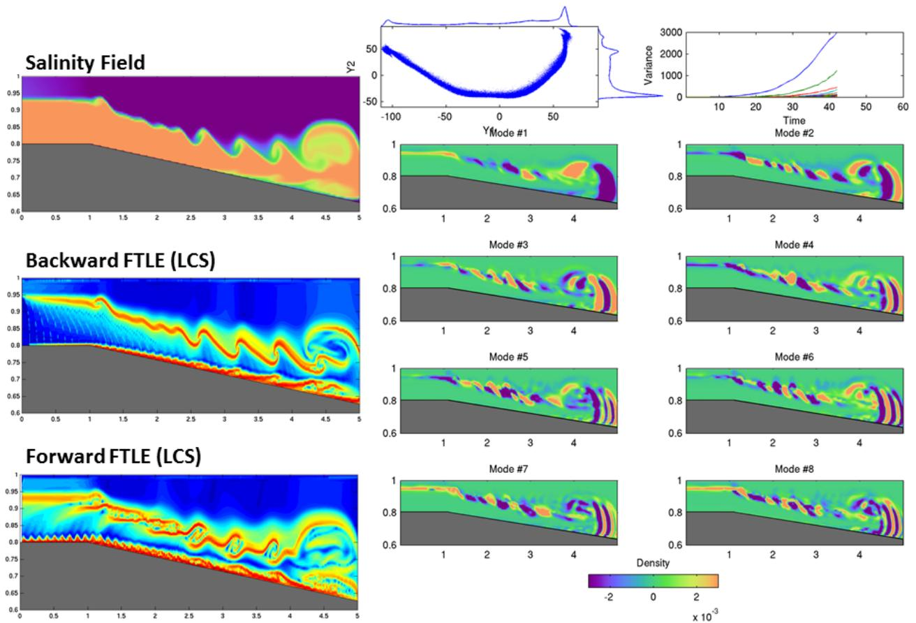
*Figure 3: Comparing LCS with DO modes for a bottom gravity current. The DO modes highlight the uncertainty in the leading edge and in the structures of the billows. The FTLE ridges also highlight these regions along with the strong flow along the bottom (where the uncertainty is low).*
