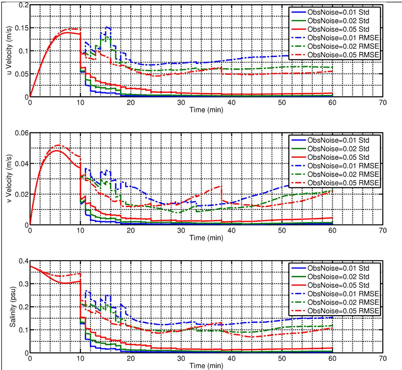
**Figure 9: Time history plots of the RMSEs and standard deviations of  $u$ ,  $v$  and salinity for three runs using the GMM-DO filter with observation standard deviation being 0.01, 0.02 and 0.05 times  $\Delta S$ , respectively.**
