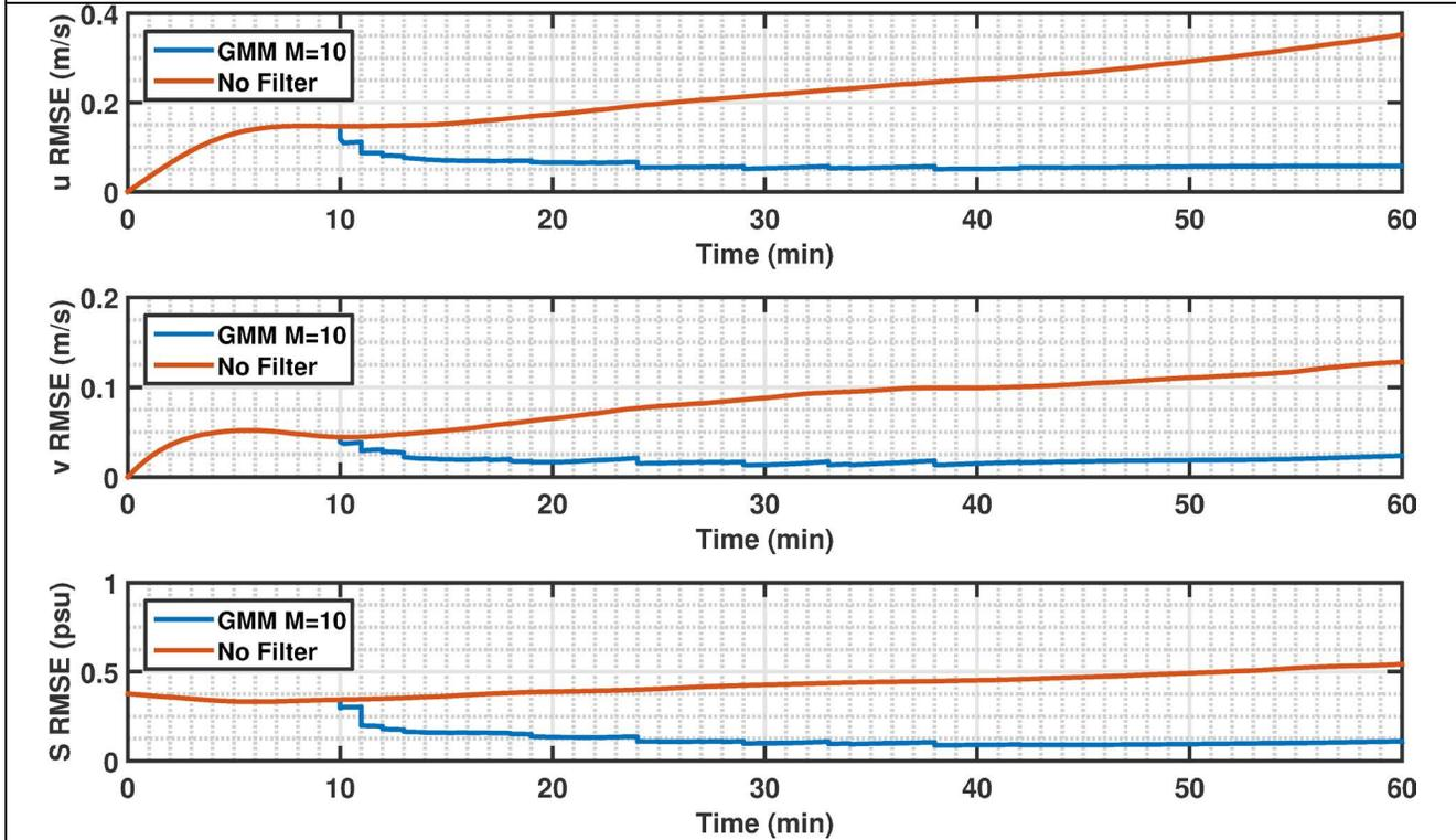
**Figure 6:** The top panel shows the DO mean, standard deviation and modes of the salinity field along with pdf's of the stochastic coefficients at non-dimensional time  $T=60$ , with no assimilation (filtering). The bottom panel shows the time history of RMSEs of  $u$ ,  $v$  and  $S$  for a stochastic run without any filtering and a run with the GMM-DO filter using 10 Gaussian components.
