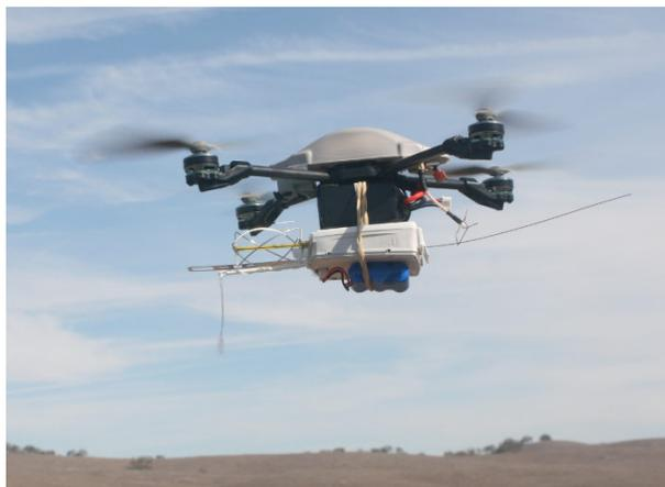
*Figure 2. The InstantEye UAV with radiosonde attached*
